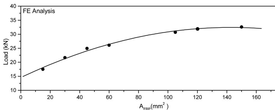
Fig. 12 Ultimate load versus area of FRPC ( $A_{FRP}$ ) laminate
