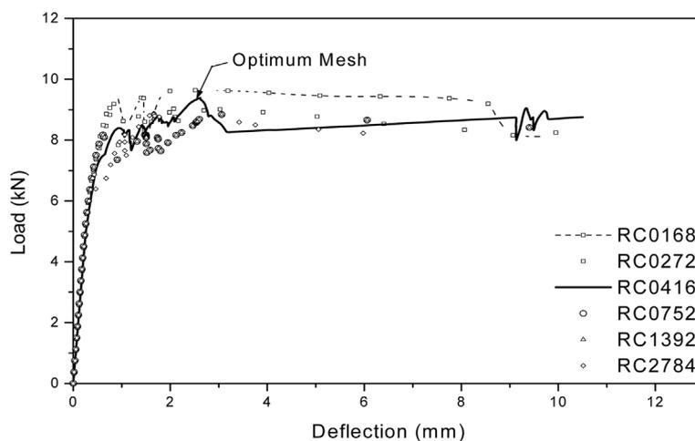
Fig. 6 Load-deflection plot for mesh convergence study (Ramana *et al.* 2000)
