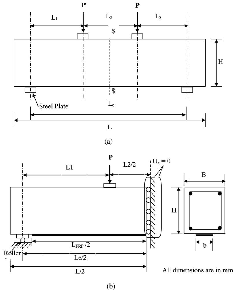
Fig. 3 Details of RC beam with FRPC
