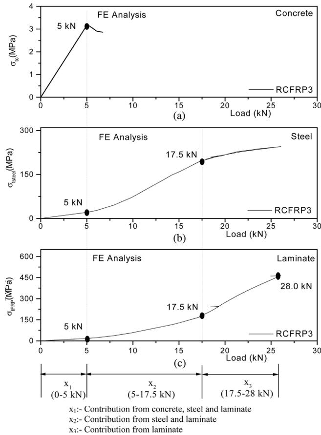
Fig. 9 Longitudinal tensile stresses in concrete ( $\sigma_{lc}$ ), laminate ( $\sigma_{IFRP}$ ) and steel reinforcement ( $\sigma_{steel}$ ) at different load levels (RCFRP3)
