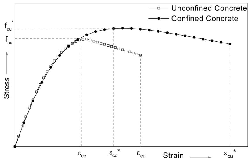
Fig. 1 Uniaxial compressive stress-strain curve for confined and unconfined concrete
