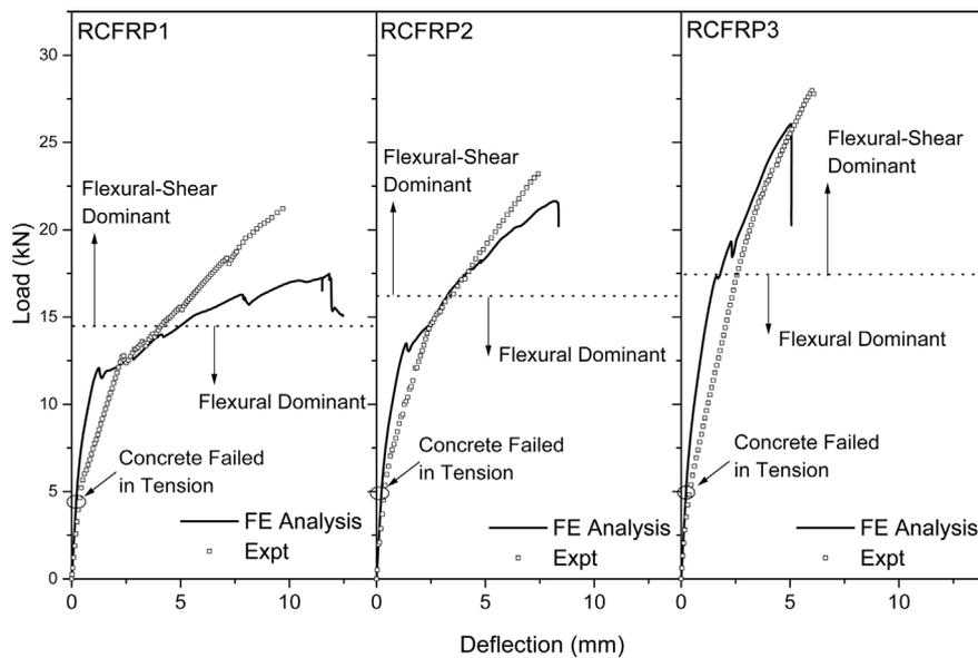
Fig 7 Load versus deflection comparison of FE analysis and experimental results (Ramana *et al.* 2000)
