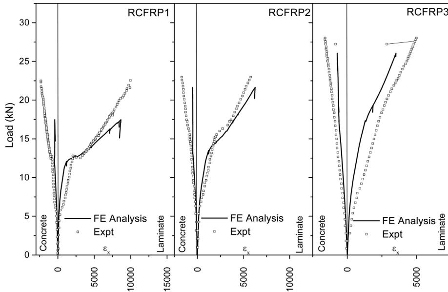
Fig 10 Load versus strain in concrete and laminate comparison of FE analysis and experimental results (Ramana *et al.* 2000)
