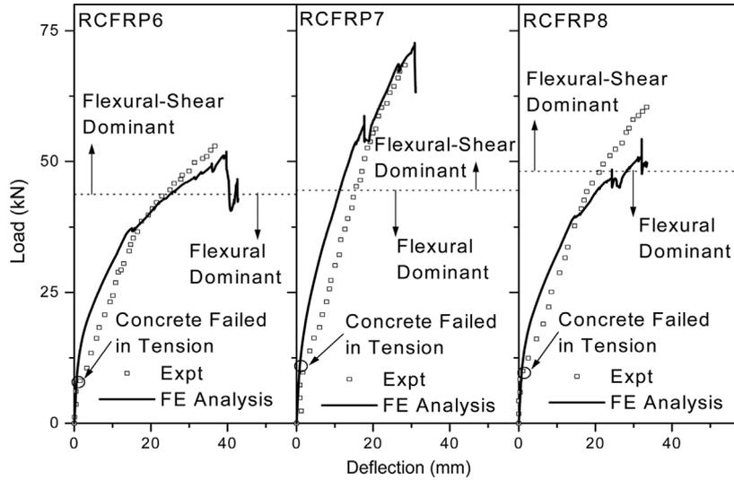
Fig 8 Load versus deflection comparison of FE analysis and experimental results (Rahimi and Hutchinson 2001)
