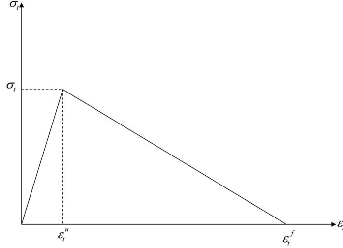
Fig. 4 Tensile stress-strain relation (Tension stiffening)
