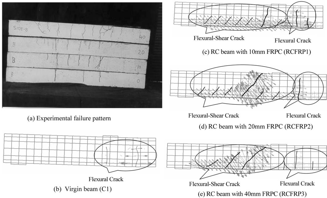
Fig. 11 Crack pattern evaluation (Ramana *et al.* 2000)
