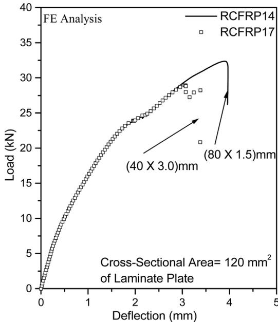
Fig. 13 Effect of ratio of width to thickness of laminate
