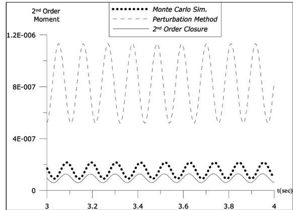
Fig. 8 Second order moment of the middle node vertical displacement
