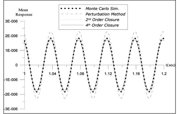
Fig. 3 Mean response of the vertical displacement of the node B
