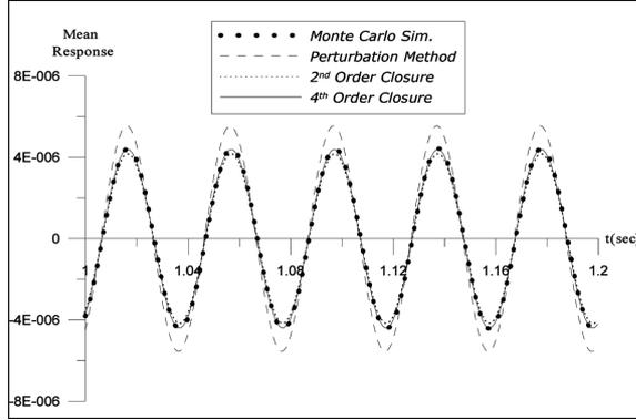
Fig. 2 Mean response of the horizontal displacement of the node A
