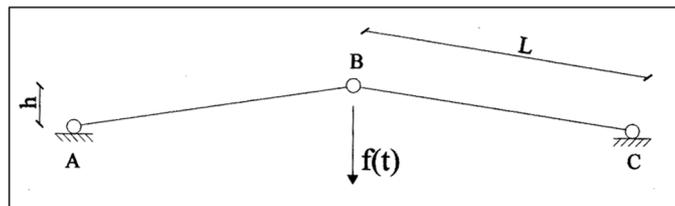
Fig. 9 Truss under examination
