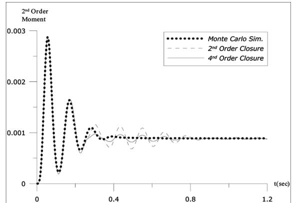
Fig. 11 Second order moment of the middle node vertical displacement
