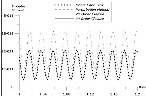
Fig. 4 Second order moment of the horizontal displacement of the node A
