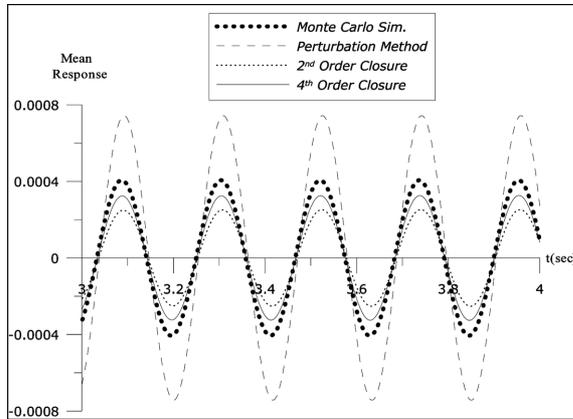
Fig. 7 Mean response of the middle node vertical displacement
