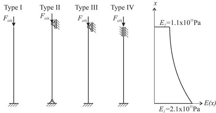
Fig. 9 Four basic types of buckling with non-constant Young’s modulus
