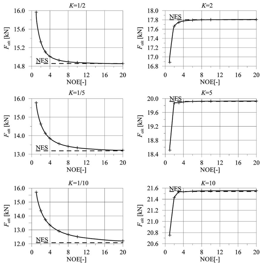
Fig. 8 Convergence of results of the Hermite beam element to our new element results – Example 4 (NES – new element solution)
