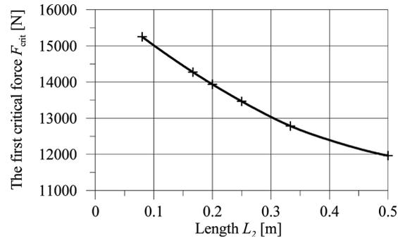
Fig. 5 The critical force dependence on length  $L_2$  (symmetric about the midspan)
