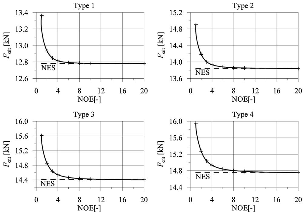
Fig. 7 Convergence of results of the Hermite beam element to our new element results – Example 3 (NES – new element solution)
