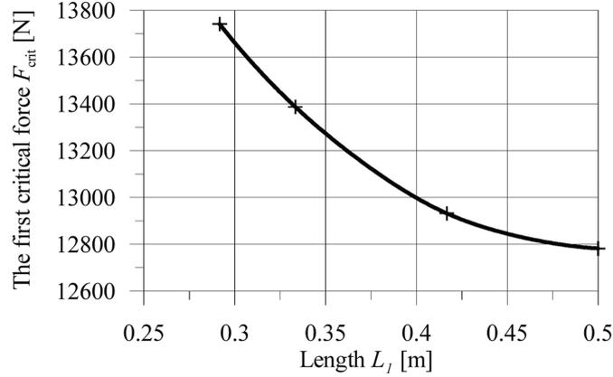
Fig. 4 The critical force dependence of length  $L_1$  – Example 1 (symmetric about the midspan)
