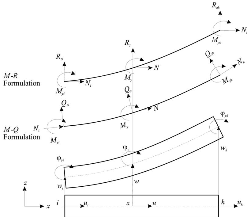
Fig. 2 Initial and deformed configuration – linearized 2nd order beam theory
