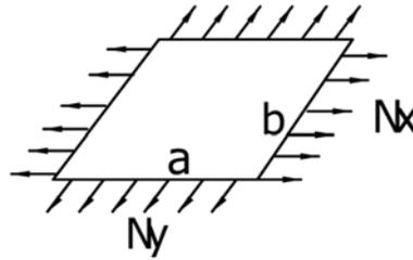
Fig. 3 A laminate subjected to bi-axis tension loads
