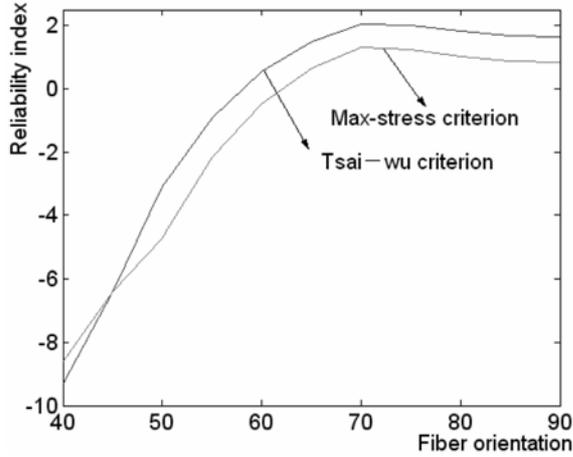
Fig. 10 Influence of different failure criteria on the reliability
