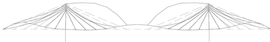
(c) Mode 3: f_3 = 0.6918 Hz (0.702 Hz)
