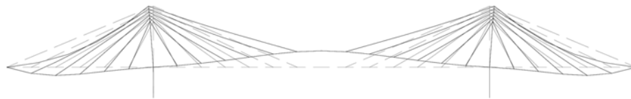
(a) Mode 1: f_1 = 0.3264 Hz (0.334 Hz)
