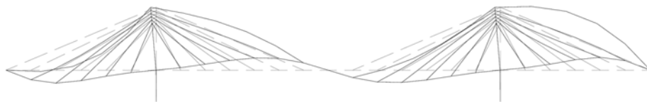
(b) Mode 2: f_2 = 0.4632 Hz (0.437 Hz)
