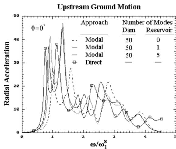
Fig. 9 Response at dam crest due to upstream ground motion by utilizing very low number of reservoir near-field modes for the pseudo-incompressible condition
