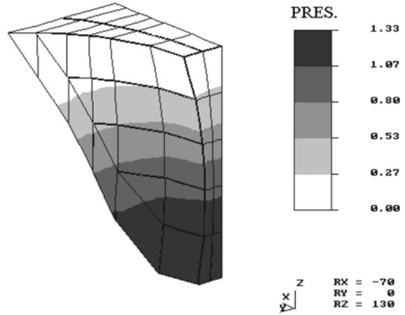
Fig. 2(b) The first mode of the reservoir near-field region
