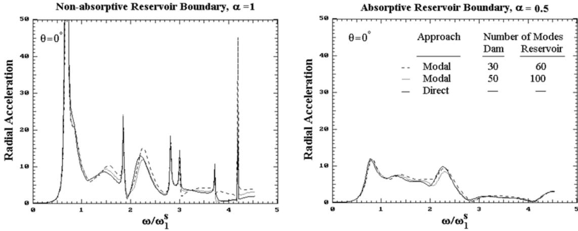
Fig. 4 Response at dam crest due to vertical ground motion
