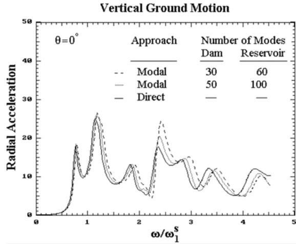
Fig. 7 Response at dam crest due to vertical excitation for the pseudo-incompressible condition
