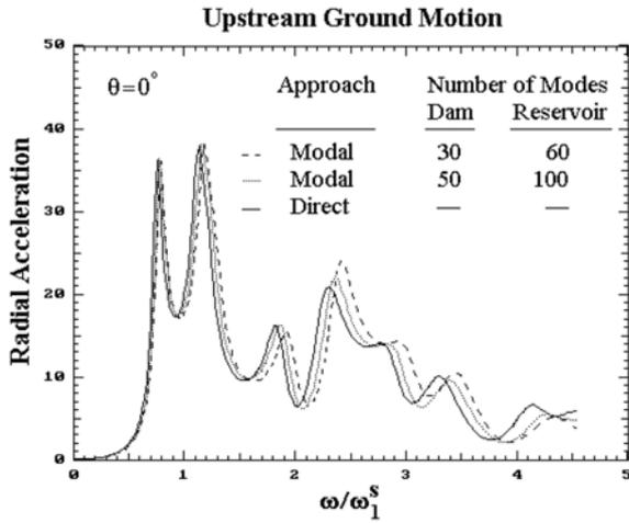
Fig. 6 Response at dam crest due to upstream excitation for the pseudo-incompressible condition
