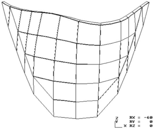
Fig. 2(a) The first decoupled mode shape of the dam on rigid foundation
