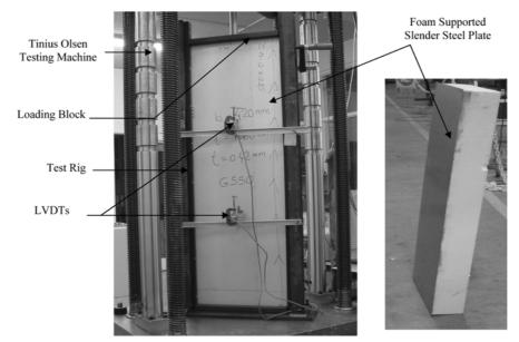
Fig. 3 Test set-up for foam-supported slender plate specimens
