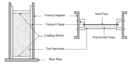
Fig. 2 Schematic diagram of test rig
