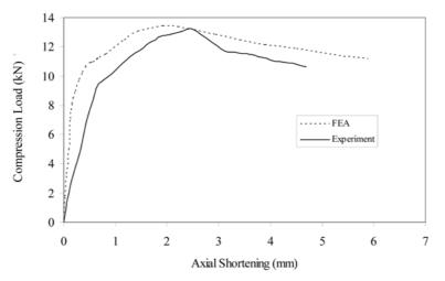
Fig. 6 Typical axial compression load versus axial shortening curve (b = 180 mm, t = 0.60 mm)
