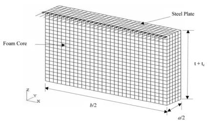
Fig. 8 Half-wave buckle length model of foam supported steel plate
