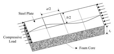
Fig. 7 Concept of half-wave buckle length model
