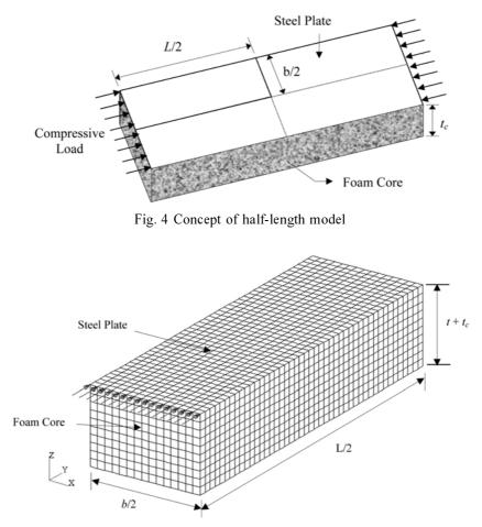
Fig. 5 Half-length model of foam supported steel plate
