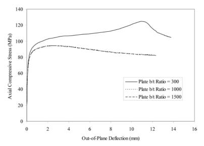
Fig. 9 Typical axial compressive stress versus out-of plane deflection
