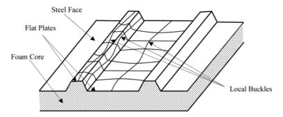
Fig. 1 Local buckling of profiled sandwich panels
