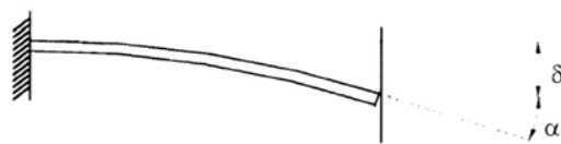
(b) Elastic deformations in a cantilever
