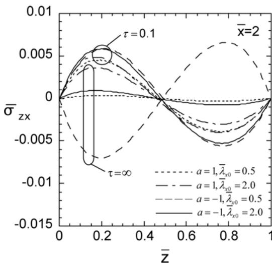
Fig. 5 Variation of shearing stress  $\bar{\sigma}_{zx}$  in the thickness direction (Case 1,  $\bar{x} = 2.0$ )
