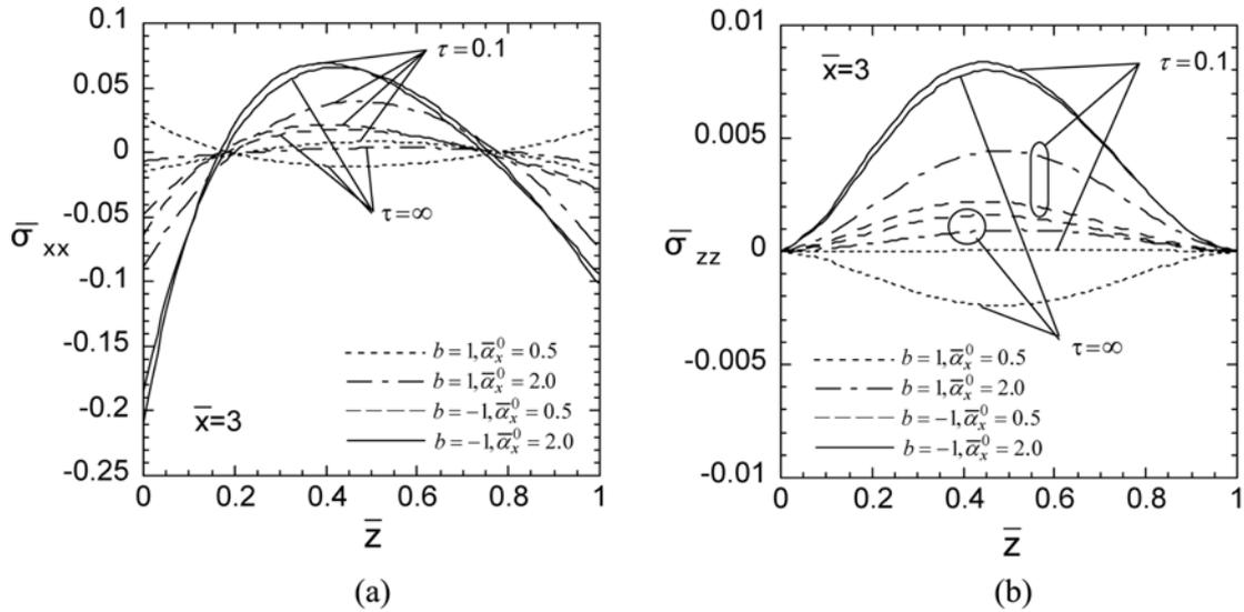
Fig. 7 Variation of thermal stress in the thickness direction (Case 2,  $\bar{x} = \bar{L}_x/2$ ); (a) Normal stress  $\bar{\sigma}_{xx}$ , (b) Normal stress  $\bar{\sigma}_{zz}$
