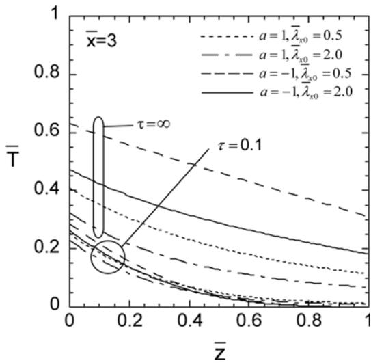
Fig. 2 Variation of temperature change in the thickness direction (Case 1,  $\bar{x} = \bar{L}_x/2$ )
