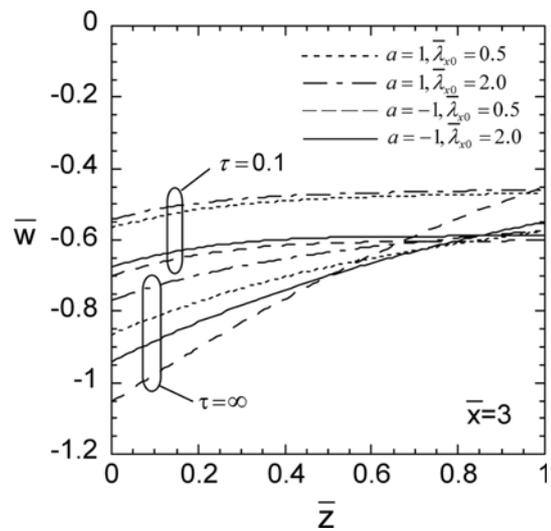
Fig. 3 Variation of thermal displacement  $\bar{w}$  in the thickness direction (Case 1,  $\bar{x} = \bar{L}_x/2$ )
