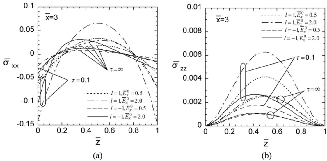
Fig. 10 Variation of thermal stress in the thickness direction (Case 3,  $\bar{x} = \bar{L}_x/2$ ); (a) Normal stress  $\bar{\sigma}_{xx}$ , (b) Normal stress  $\bar{\sigma}_{zz}$
