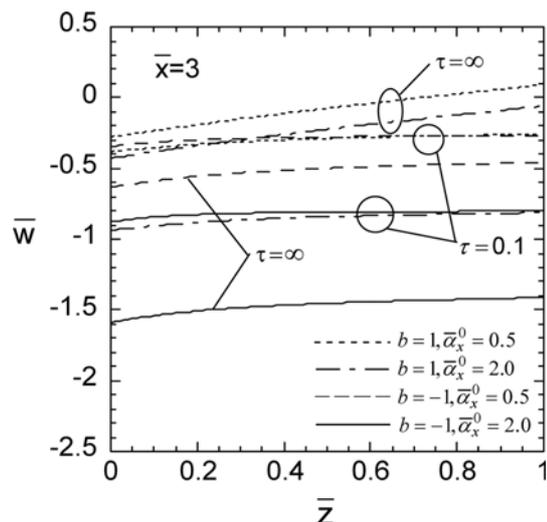
Fig. 6 Variation of thermal displacement  $\bar{w}$  in the thickness direction (Case 2,  $\bar{x} = L_x/2$ )
