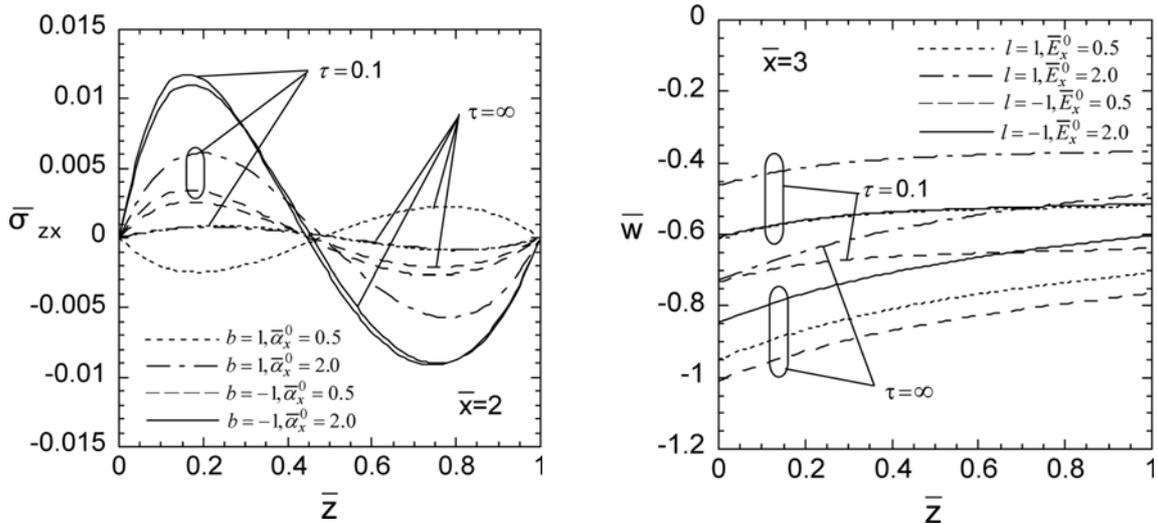
Fig. 8 Variation of shearing stress  $\bar{\sigma}_{zx}$  in the thickness direction (Case 2,  $\bar{x} = 2.0$ )
