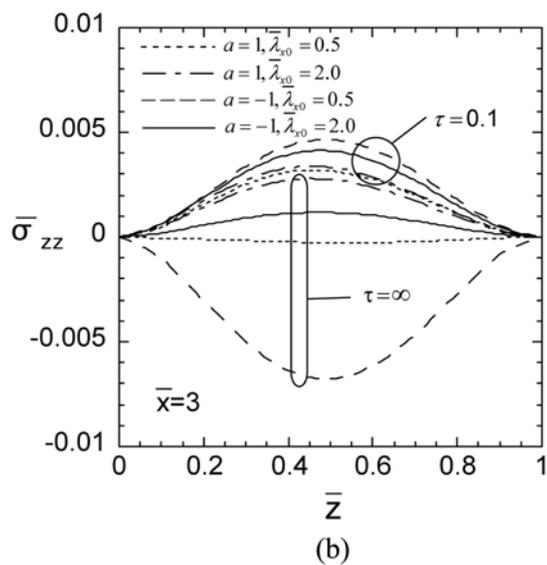
Fig. 4 Variation of thermal stress in the thickness direction (Case 1,  $\bar{x} = \bar{L}_x/2$ ); (a) Normal stress  $\bar{\sigma}_{xx}$ , (b) Normal stress  $\bar{\sigma}_{zz}$
