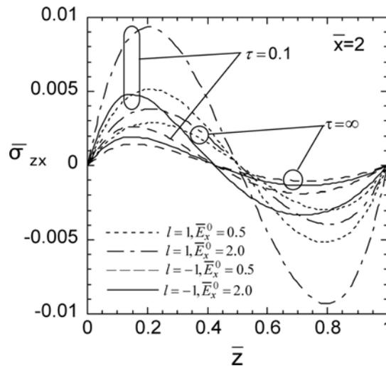
Fig. 11 Variation of shearing stress  $\bar{\sigma}_{zx}$  in the thickness direction (Case 3,  $\bar{x} = 2.0$ )
