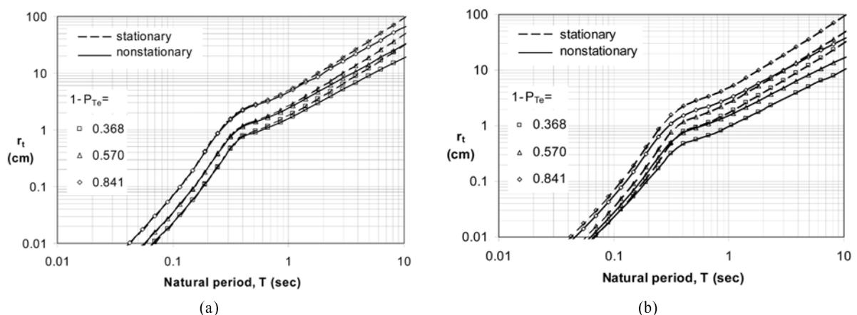
Fig. 1 Peak responses of SDOF systems to the evolutionary Kanai-Tajimi PSD function. (a) Boxcar modulating function, (b) Exponential modulating function
