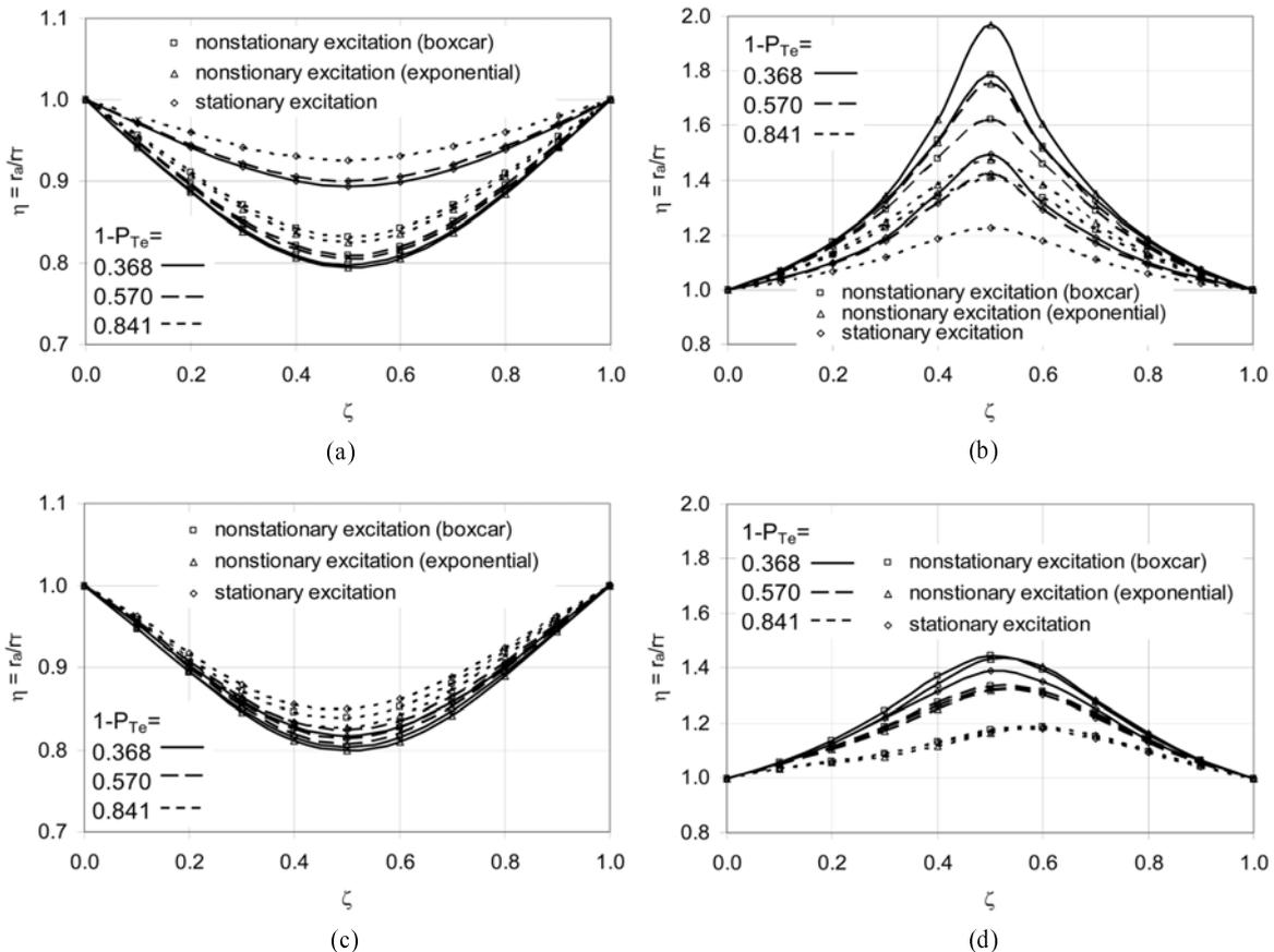
Fig. 5 Comparison between the ratios of stationary cases and nonstationary cases (with the Kanai-Tajimi PSD function). (a)  $T_1 = 0.2s$ ,  $T_1/T_2 = 1.2$ ,  $\text{sgn}(C_1C_2) > 0$ , (b)  $T_1 = 0.2s$ ,  $T_1/T_2 = 1.2$ ,  $\text{sgn}(C_1C_2) < 0$ , (c)  $T_1 = 0.2s$ ,  $T_1/T_2 = 2.0$ ,  $\text{sgn}(C_1C_2) > 0$ , (d)  $T_1 = 0.2s$ ,  $T_1/T_2 = 2.0$ ,  $\text{sgn}(C_1C_2) < 0$
