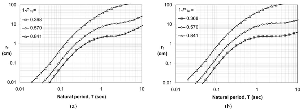
Fig. 2 Peak responses of SDOF systems to the evolutionary PSD function of seismological model. (a) Boxcar modulating function, (b) Exponential modulating function
