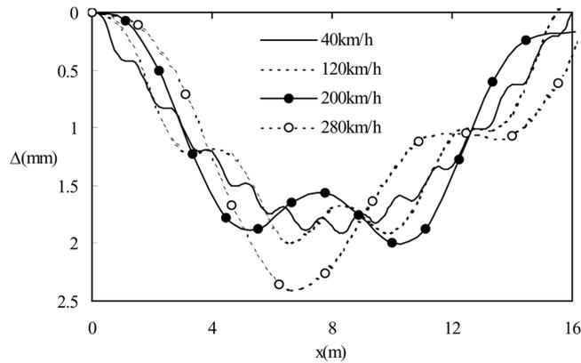
Fig. 3 Response of mid-span deflection to the vehicle position
