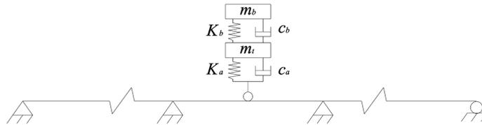
Fig. 2 The interaction model of vehicle-bridge system
