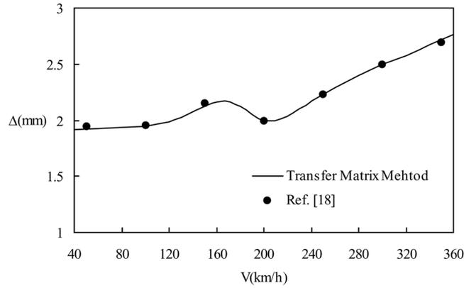
Fig. 4 Response of maximum mid-span deflection to the vehicle velocity
