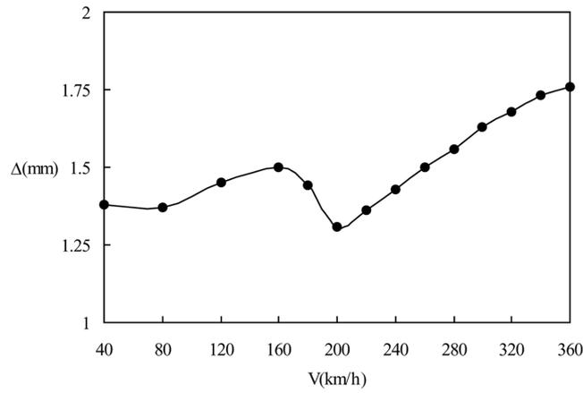
Fig. 7 Response of maximum mid-span deflection to the vehicle velocity
