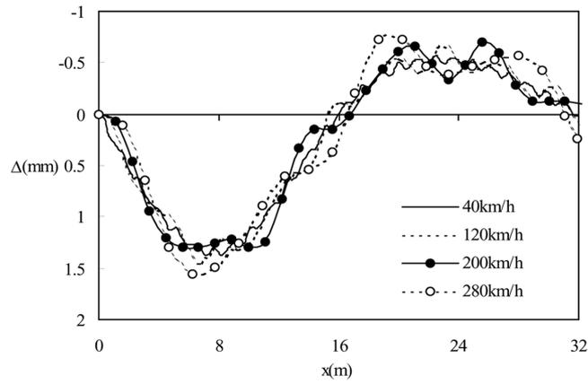
Fig. 6 Response of mid-span deflection to the vehicle position
