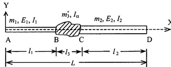
Fig. 1 Notation and coordinate system of a two-part beam-mass system for the transfer matrix method
