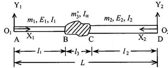
Fig. 3 Notation and coordinate system of a two-part beam-mass system for the direct method
