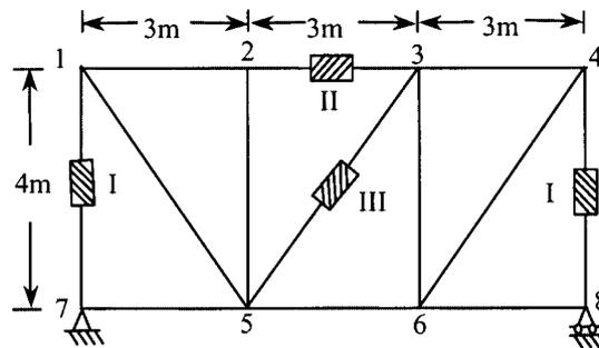
Fig. 5 A framework consisting of two-part beam-mass systems with nodes 1 to 8 and member types I, II and III
