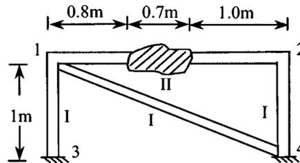
Fig. 4 A framework consisting of two-part beam-mass systems with nodes 1 to 4, and member types I and II
