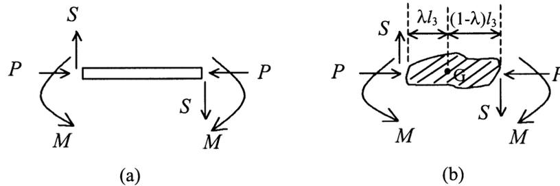
Fig. 2 Sign convention for positive axial force ( $P$ ), shear force ( $S$ ) and bending moment ( $M$ ) (a) for a beam element, (b) for a rigid mass element
