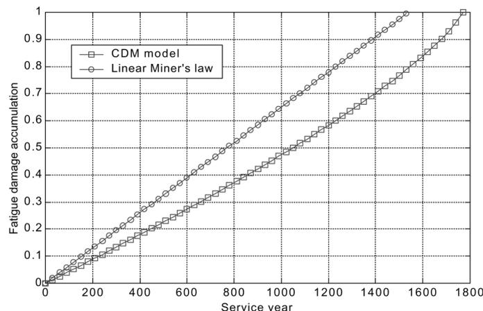
Fig. 14 Fatigue damage accumulation at the location of SSTLN-01 using nominal stress approach
