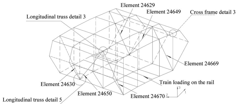
Fig. 4 The typical deck element
