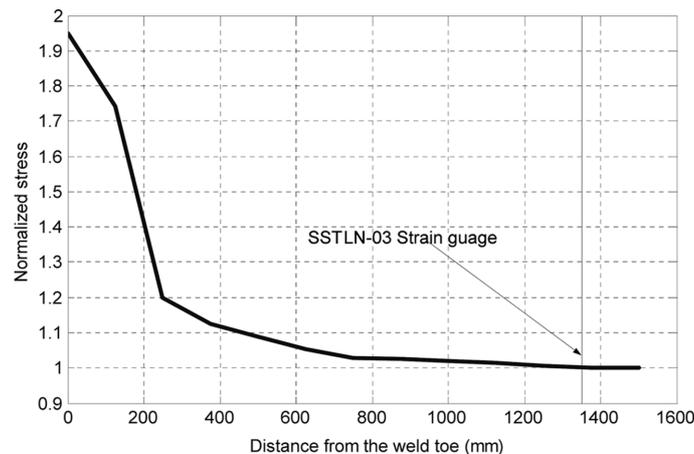
Fig. 11 Stress distribution along the longitudinal truss detail 5
