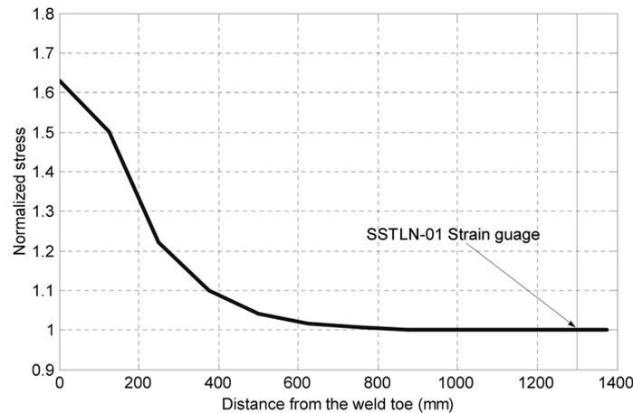
Fig. 10 Stress distribution along the longitudinal truss detail 3
