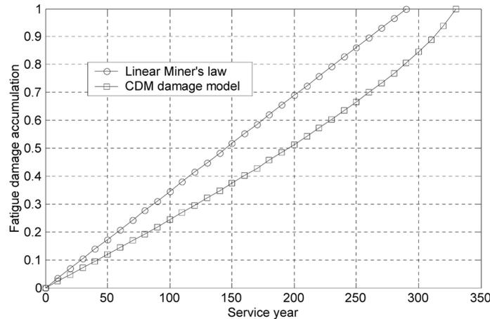
Fig. 15 Fatigue damage accumulation at the location of SSTLN-01 using hot spot stress approach
