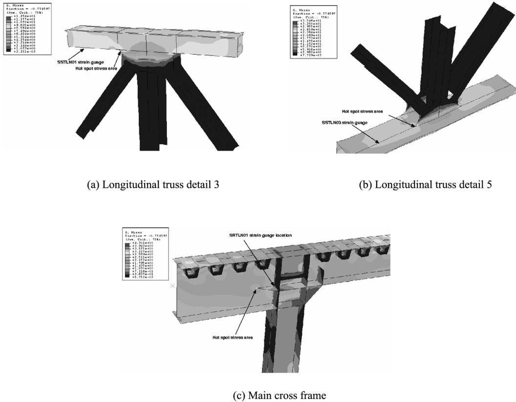
Fig. 9 Stress distribution for various joint details
