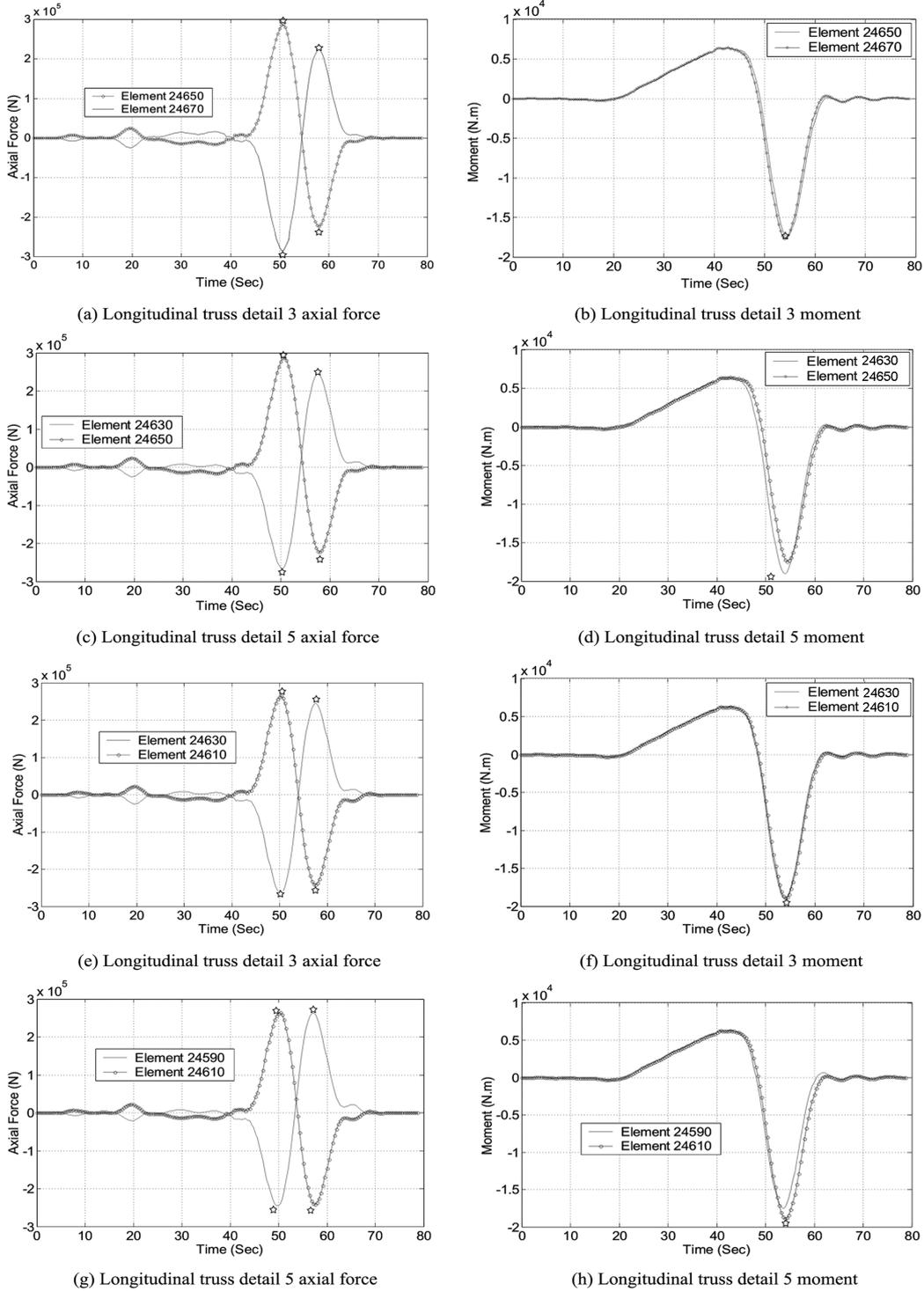
Fig. 8 Internal forces of longitudinal truss under train loading
