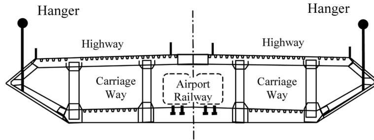
Fig. 2 Typical deck section of the Tsing Ma Bridge
