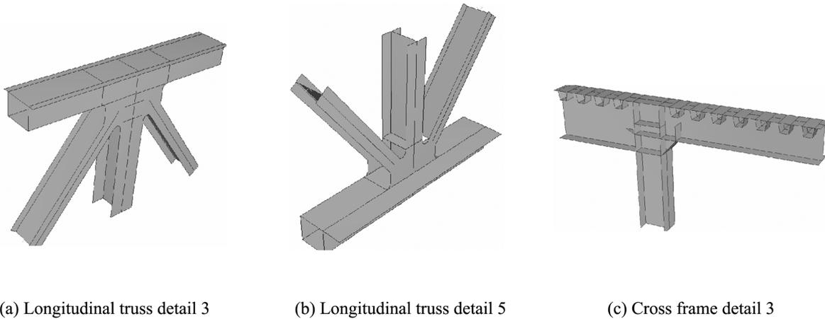
Fig. 5 Joint geometry of typical deck investigated
