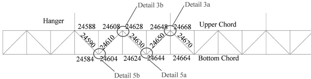
Fig. 6 Longitudinal truss element number of a typical longitudinal truss
