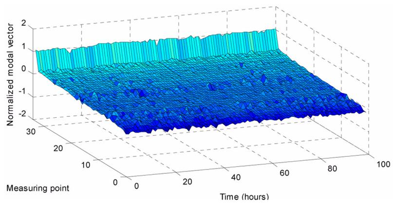
Fig. 13 Variability of measured modal vectors for the second mode
