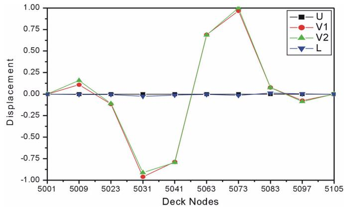
Fig. 7 Identified shape of the first mode ( $f_1 = 0.165$  Hz)
