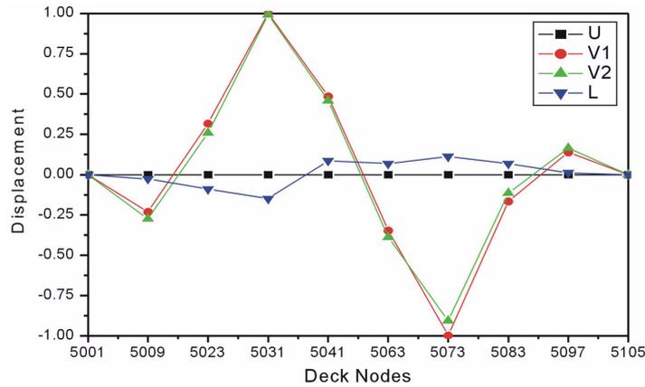
Fig. 11 Identified shape of the fifth mode ( $f_5 = 0.300$  Hz)
