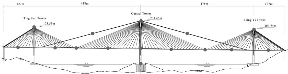
Fig. 3 Elevation of Ting Kau Bridge
