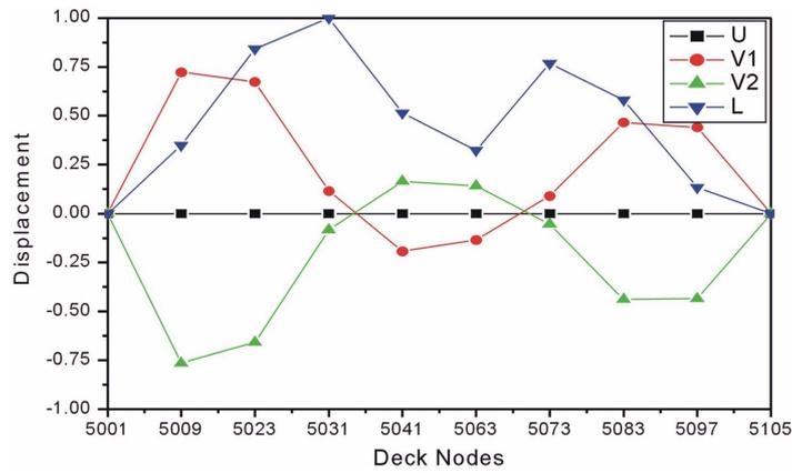
Fig. 10 Identified shape of the fourth mode ( $f_4 = 0.291$  Hz)
