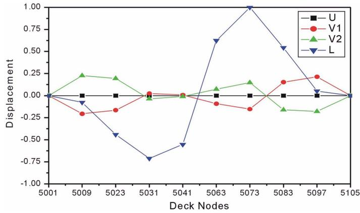
Fig. 9 Identified shape of the third mode ( $f_3 = 0.264$  Hz)
