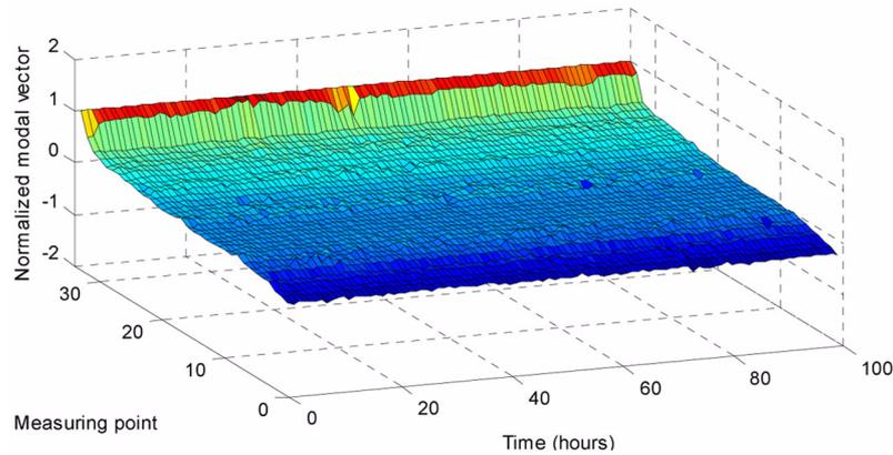
Fig. 15 Variability of measured modal vectors for the fourth mode
