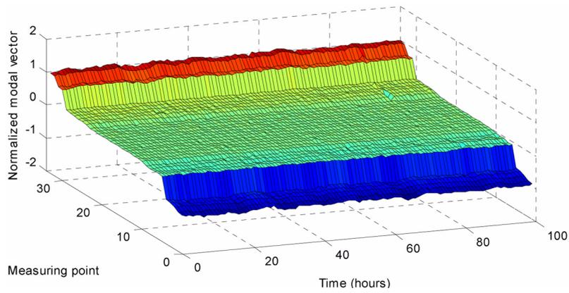
Fig. 12 Variability of measured modal vectors for the first mode
