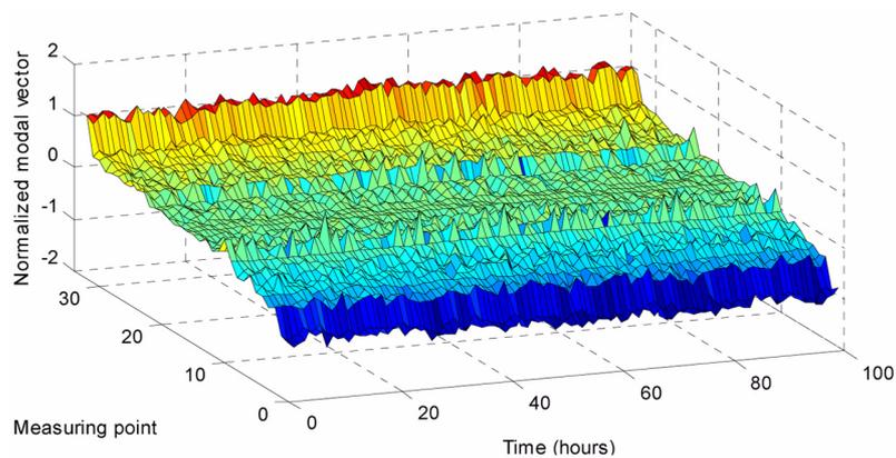
Fig. 16 Variability of measured modal vectors for the fifth mode
