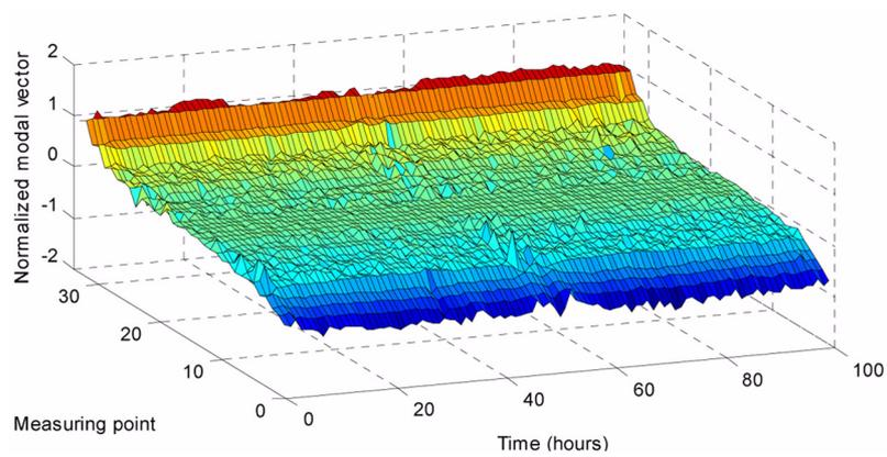
Fig. 14 Variability of measured modal vectors for the third mode
