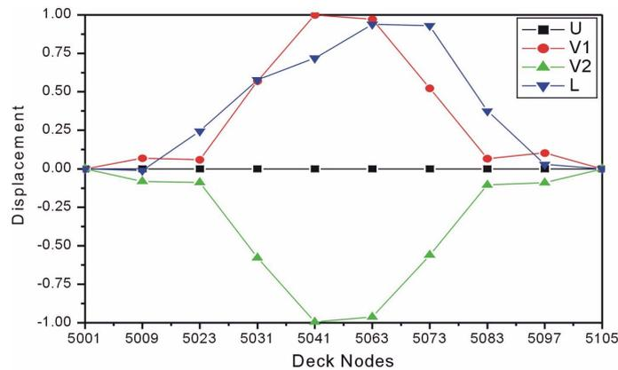
Fig. 8 Identified shape of the second mode ( $f_2 = 0.228$  Hz)
