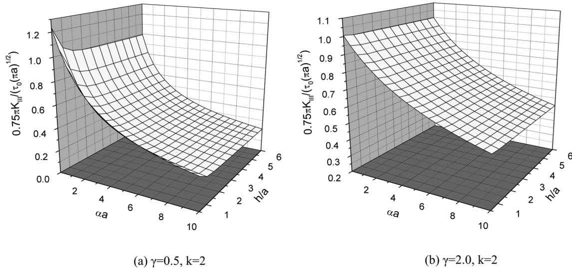
Fig. 5 The relation of normalized stress intensity factor  $0.75\pi K_{III}/\tau_0(\pi a)^{1/2}$  with  $h/a$  and  $\alpha a$
