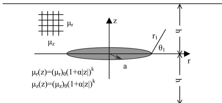
Fig. 1 Penny-shaped crack in transversely isotropic functionally graded strip
