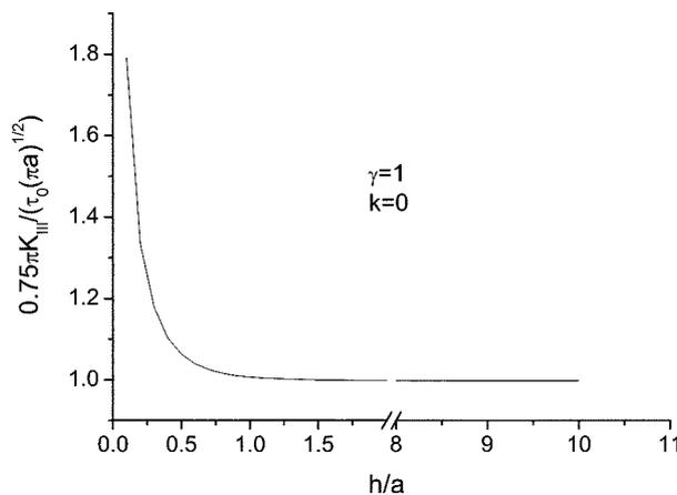
Fig. 2 Normalized stress intensity factor  $0.75\pi K_{III} / \tau_0(\pi a)^{1/2}$  with  $h/a$  for isotropic homogeneous strip
