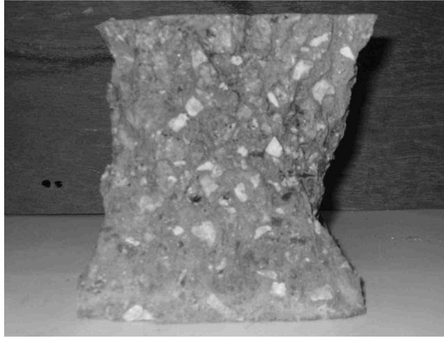
Fig. 14 Typical failure of concrete cube under compressive loading
