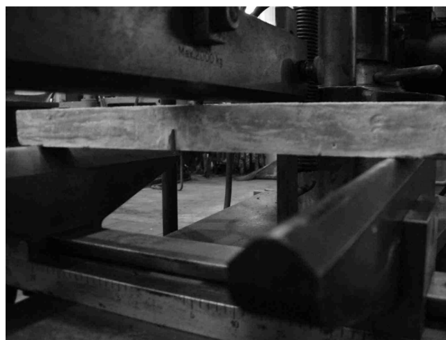
Fig. 11 Test setup for evaluating fracture toughness of mortar
