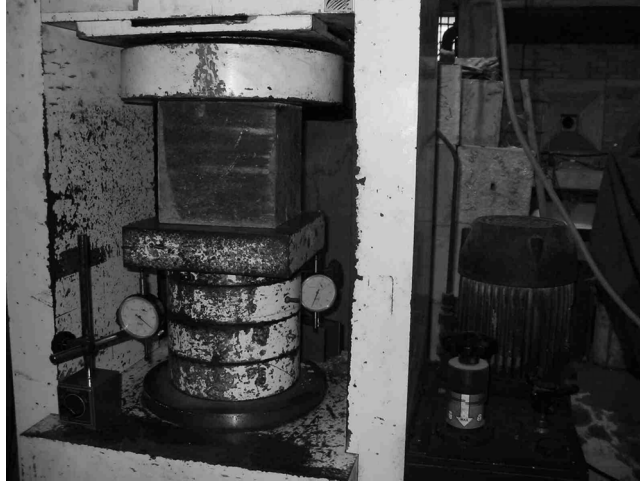
Fig. 12 Test setup for compressive test of concrete cube
