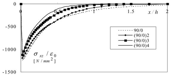
(a) interlaminar shear stress at upper 0/90 interface
