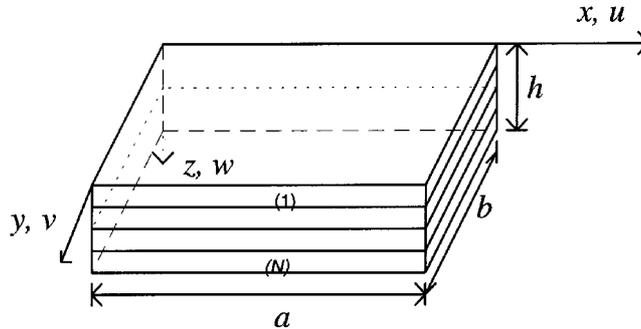
Fig. 1 Nomenclature of a laminated rectangular plate
