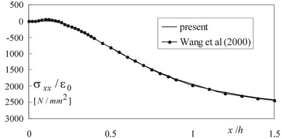
(b) in-plane stress at the middle interface of the laminate
