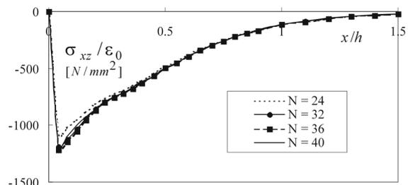
(a) interlaminar shear stress at 0/90 interface
