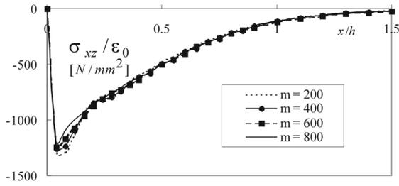
(a) interlaminar shear stress at 0/90 interface
