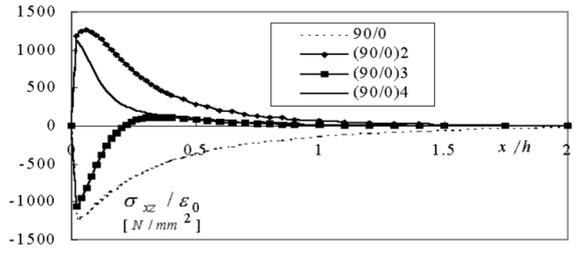
(a) interlaminar shear stress at middle surface of the laminate
