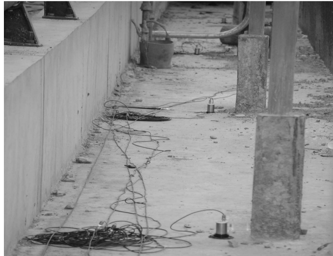
Fig. 8 Photo of vertical accelerometers installed on the bridge deck
