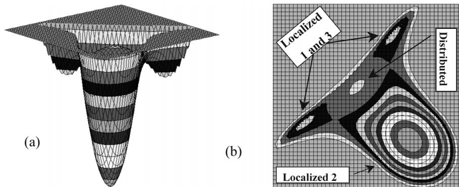
Fig. 2 The energy variation of the three-bar truss (for Case 1). (a) The energy profile close to the extremum points; (b) The contour plot of the locality close to the extremum points
