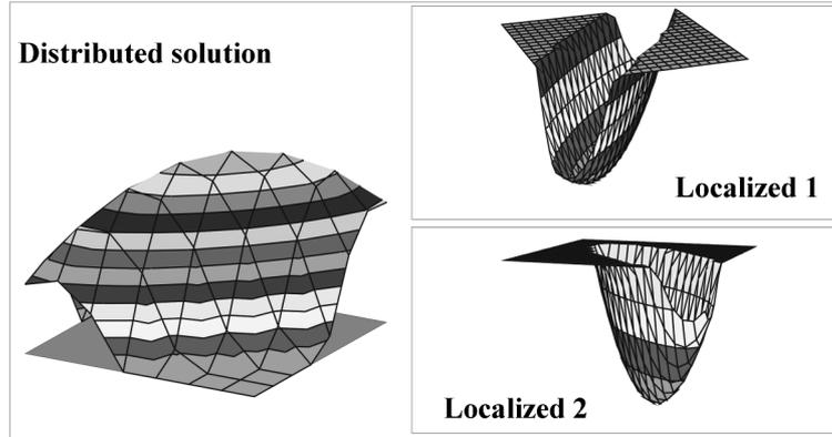
Fig. 3 The energy variation of the three-bar truss close to the extremum points (for Case 2)
