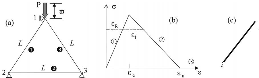
Fig. 1 (a) A three-bar truss, (b) Constitutive law, (c) Bar element
