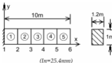
Fig. 1 The cantilever beam structure
