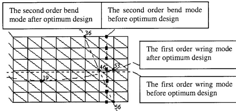
Fig. 4 The position of node line of plate structure before and after optimum design
