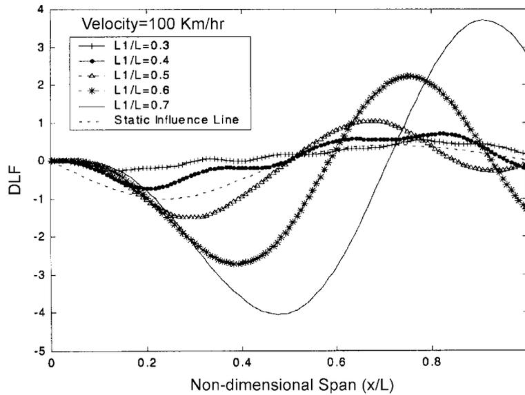
Fig. 5(a) DLF at the midpoint of the first span versus nondimensional span for various the first span lengths
