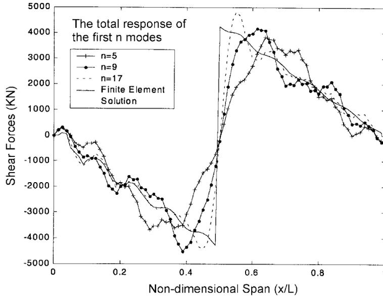
Fig. 1(c) Influence lines of shear force of the simply supported Beam at the midspan
