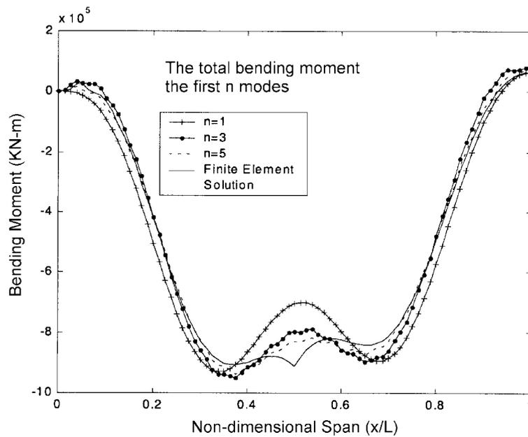
Fig. 1(b) Influence lines of bending moment of the simply supported beam at the midspan
