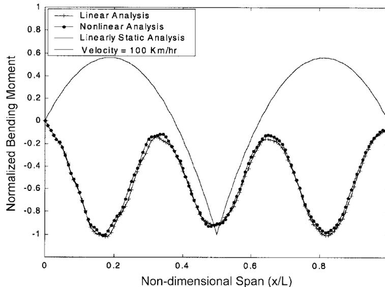
Fig. 6(c) Nonlinear effect on bending moment
