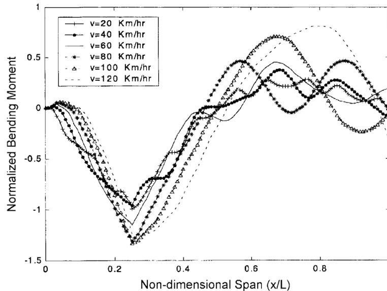
Fig. 3(c) Normalized bending moment  $M^*$  at the midpoint of the first span versus non-dimensional span ( $x/L$ ) for various velocities
