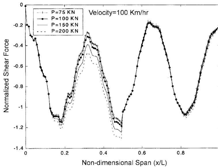
Fig. 4(b) Normalized shear  $V^*$  of realistic loading conditions at the internal support versus nondimensional span  $(x/L)$  for various velocities
