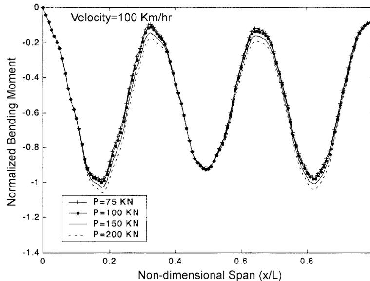
Fig. 4(c) Normalized bending moment  $M^*$  of realistic loading conditions at the midpoint of the first span versus nondimensional span ( $x/L$ ) for various velocities
