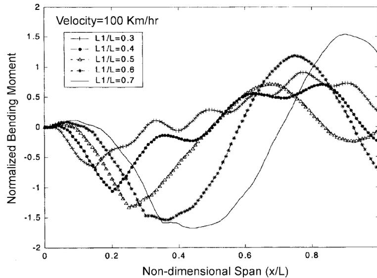
Fig. 5(c) Normalized bending moment at the midpoint of the first span versus span for various the first span lengths
