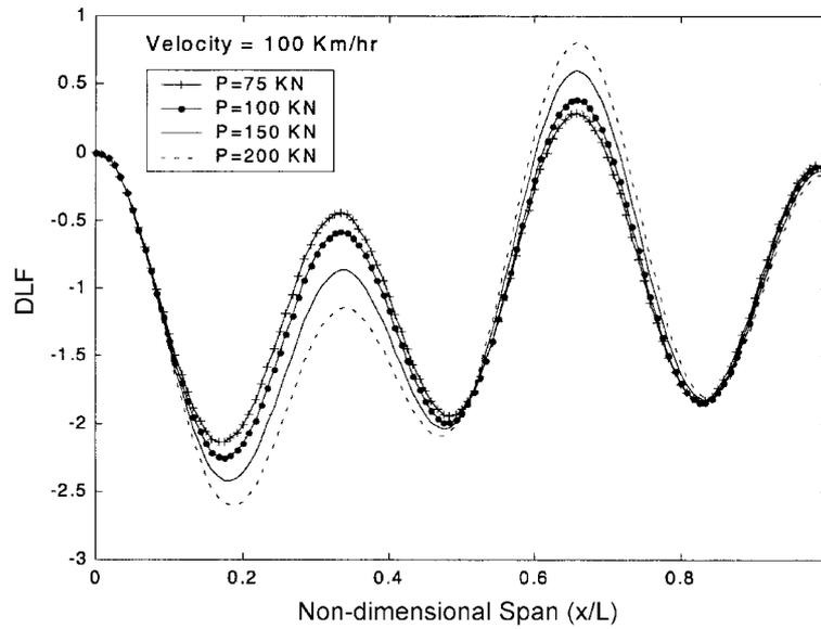
Fig. 4(a) Nondimensional span versus DLF of realistic loading conditions at the midpoint of the first span for various velocities
