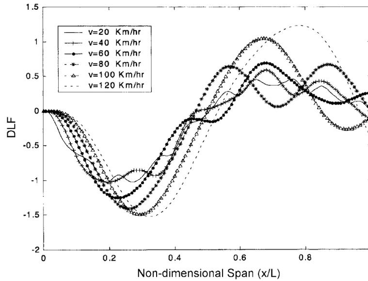
Fig. 3(a) Nondimensional span versus DLF at the midpoint of the first span for various velocities
