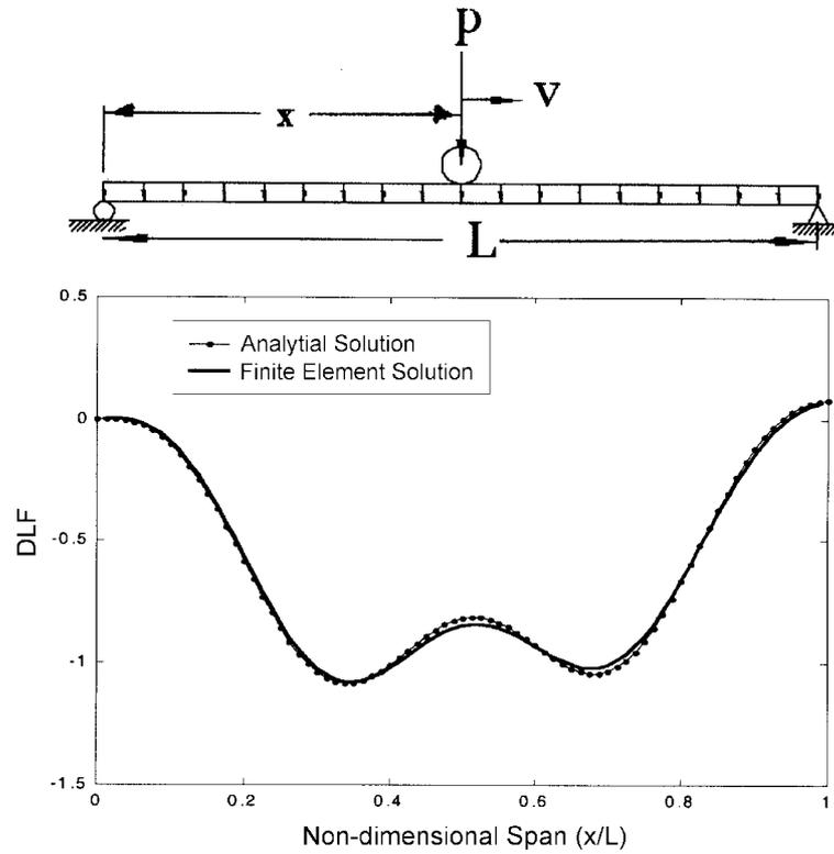
Fig. 1(a) DLF of the simply supported beam subjected to a moving load at the midspan
