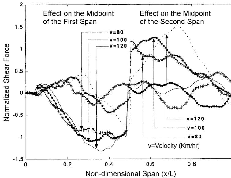
Fig. 3(b) Normalized shear  $V^*$  versus non-dimensional span ( $x/L$ ) for various velocities at the midpoint of the first span
