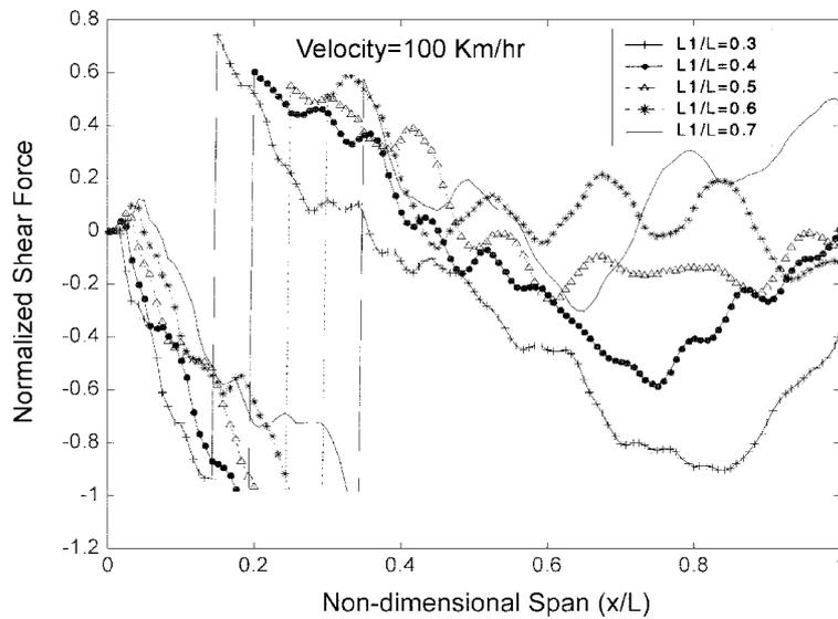
Fig. 5(b) Normalized shear force versus span for different span lengths
