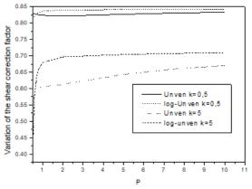
Fig. 14 Effect of the type of porosity distribution uneven and Log-uneven of FGP beam on shear correction for  $E_t/E_b=4$  and  $\xi=0.2$
