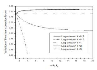
Fig. 8 Variation of the shear correction factor according to  $n = E_t/E_b$  and the power law index k for the FG beam Log-uneven p = 0.5 and  $\xi = 0.2$
