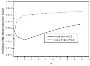
Fig. 15 Effect of the type of porosity distribution uneven and Log-uneven of FGP beam on shear correction for  $E_t/E_b=4$ , k=0.5 and  $\xi=0.2$
