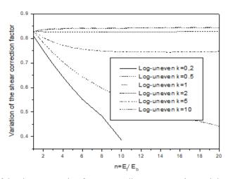
Fig. 9 Variation of the shear correction factor according to  $n = E_t/E_b$  and the power law index k for the FG beam Log-uneven p = 5 and  $\xi = 0.2$
