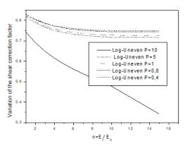
Fig. 13 Variation of the shear correction factor according to  $n = E_t/E_b$  and the porosity parameter p for the FG beam Log-uneven k = 2 and  $\xi = 0.2$
