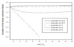
Fig. 6 Variation of the shear correction factor according to  $n = E_t/E_b$  and the power law index k for the FG beam uneven p = 0.5 and  $\xi = 0.2$
