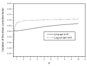
Fig. 16 Effect of the type of porosity distribution uneven and Log-uneven of FGP beam on shear correction for  $E_t/E_b=4$ , k=5 and  $\xi=0.2$
