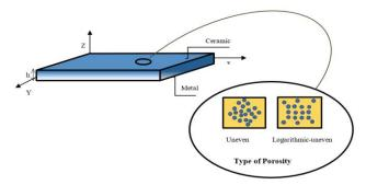
Fig. 1 Model of functionally graded porous beam
