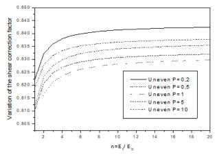
Fig. 10 Variation of the shear correction factor according to  $n = E_t/E_b$  and the porosity parameter p for the FG beam uneven k = 0.5 and  $\xi = 0.2$
