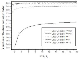
Fig. 12 Variation of the shear correction factor according to  $n = E_t/E_b$  and the porosity parameter p for the FG beam Log-uneven k = 0.5 and  $\xi = 0.2$
