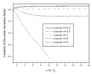
Fig. 7 Variation of the shear correction factor according to  $n = E_t/E_b$  and the power law index k for the FG beam uneven p = 5 and  $\xi = 0.2$
