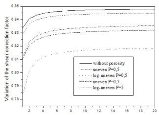
Fig. 4 Comparaison of Variation of the shear correction factor for the FG beam without porosity and two types of porosity (uneven, Log-unven) for p = 0.5
