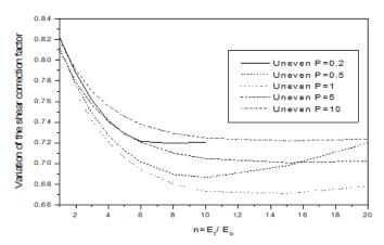
Fig. 11 Variation of the shear correction factor according to  $n = E_t/E_b$  and the porosity parameter p for the FG beam uneven k = 2 and  $\xi = 0.2$
