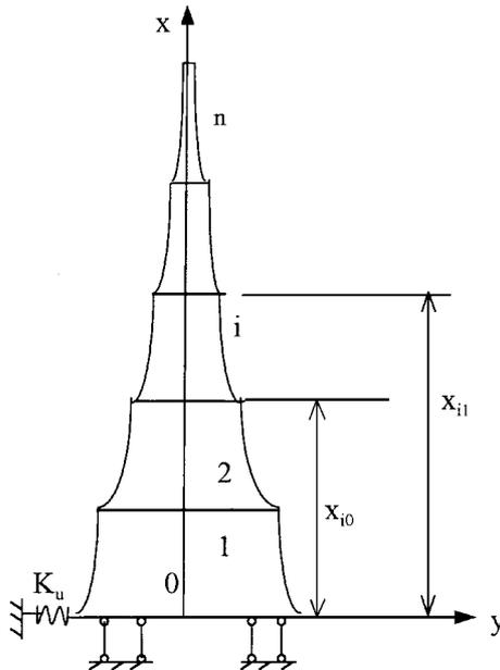
Fig. 4 A multi-step free-spring supported shear beam
