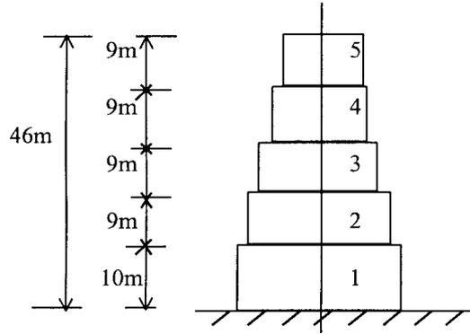
Fig. 6 The five-step beam model of the building
