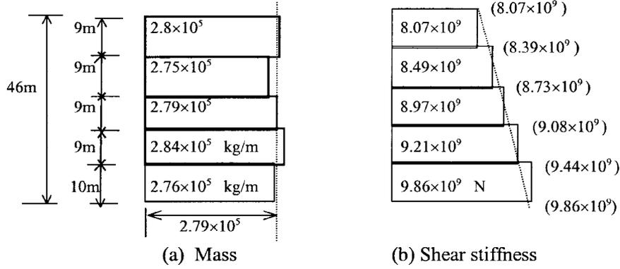
Fig. 5 The distributions of mass and stiffness of the building
