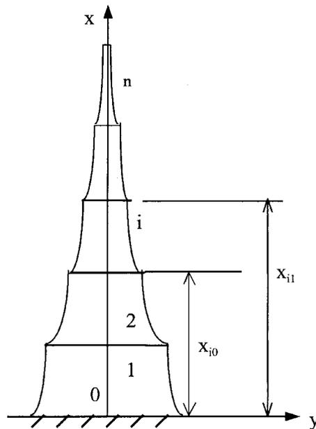
Fig. 3 A multi-step shear beam
