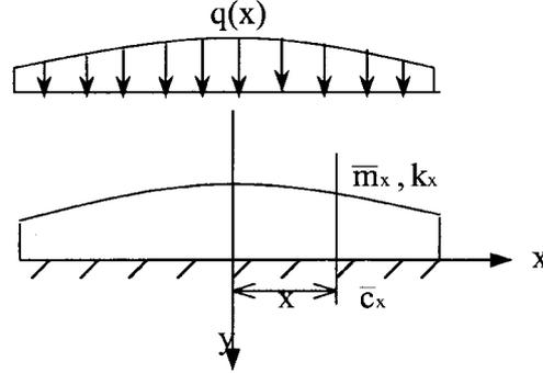
Fig. 1 A shear beam on an elastic foundation
