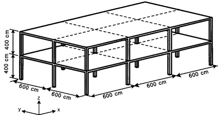
Fig. 4 Example structure with many slabs
