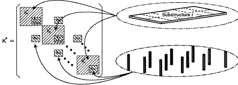
Fig. 11 Construction of stiffness matrix for global system
