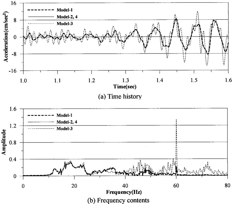
Fig. 17 Acceleration responses at node B
