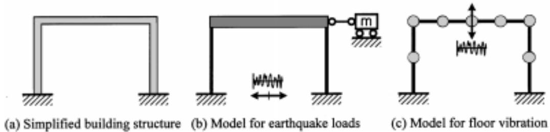
Fig. 1 Analytical modeling of a building structure
