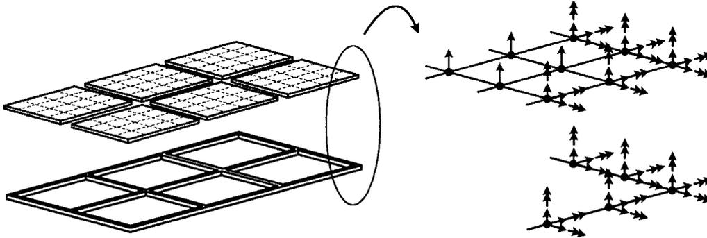
Fig. 10 Substructure modeled as a super element
