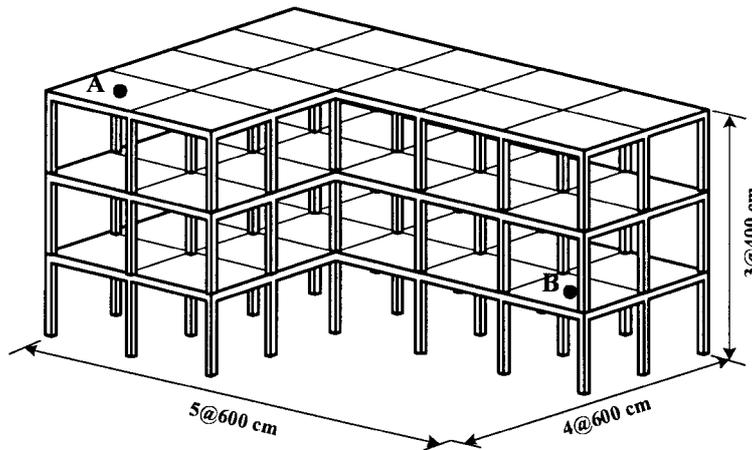
Fig. 18 Analysis model for unsymmetric building structure
