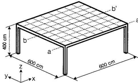
Fig. 6 8x8 finite element division of slab
