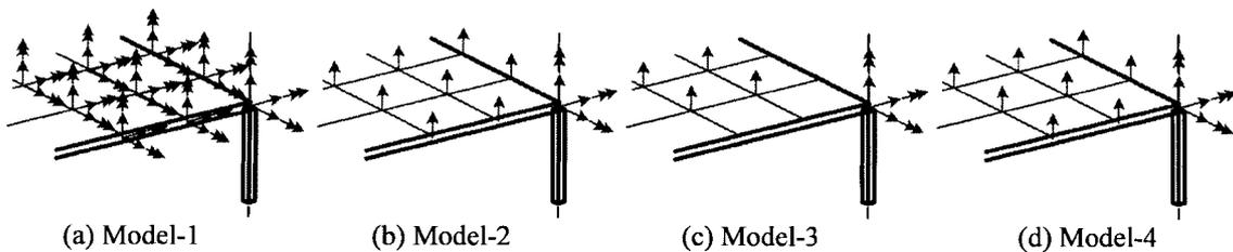
Fig. 14 Selected master DOF’s for the example structure
