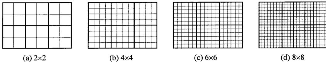
Fig. 5 Mesh division for floor vibration analysis
