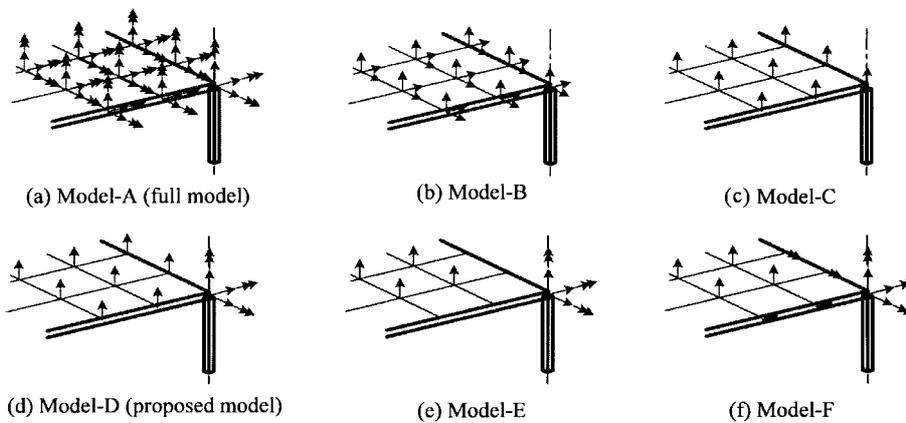
Fig. 8 Selected master DOF's for various selection criteria
