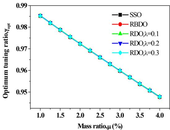
Fig. 4 The optimum tuning ratio with increasing mass ratio
