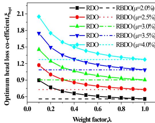
Fig. 9 The optimum head loss coefficient with varying weight factor,  $\lambda$  for different mass ratio
