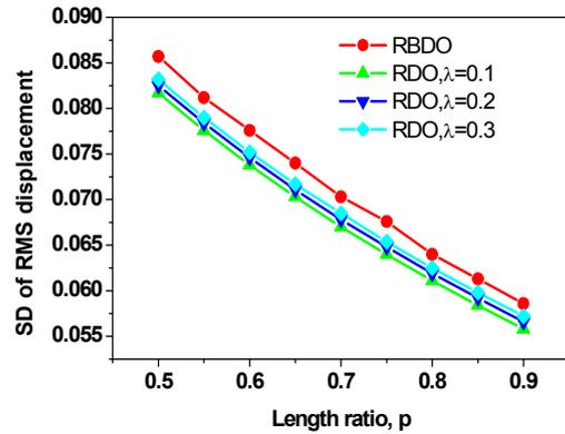
Fig. 15 The variation of the SD of the rmsd of the primary structure with varying length ratio
