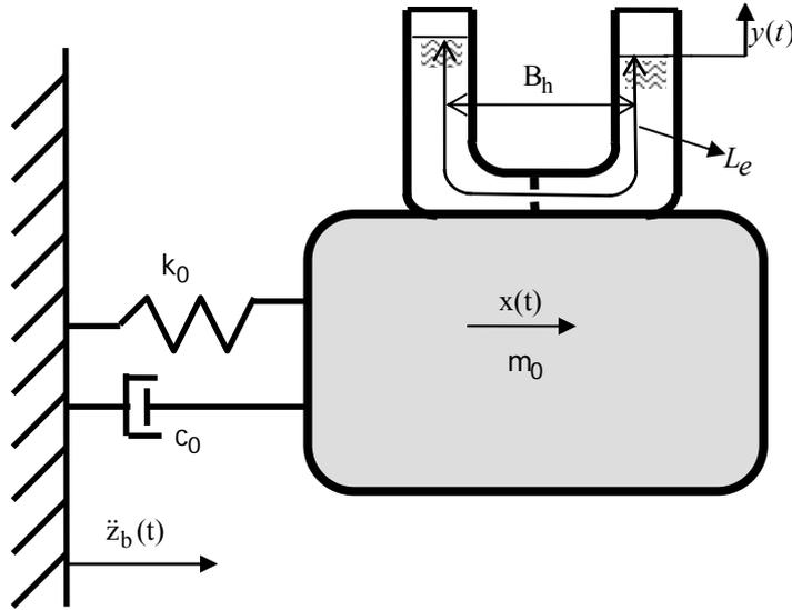
Fig. 1 The liquid column vibration absorbers model
