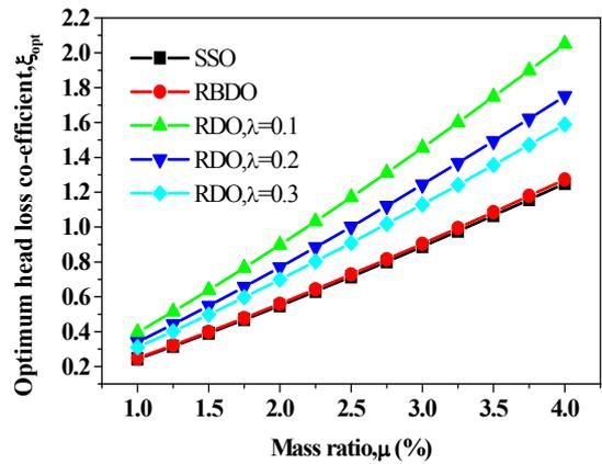
Fig. 5 The optimum head loss coefficient with increasing mass ratio
