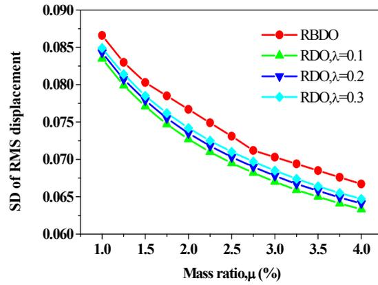
Fig. 3 The variation of the SD of the rmsd of the primary structure with increasing mass ratio
