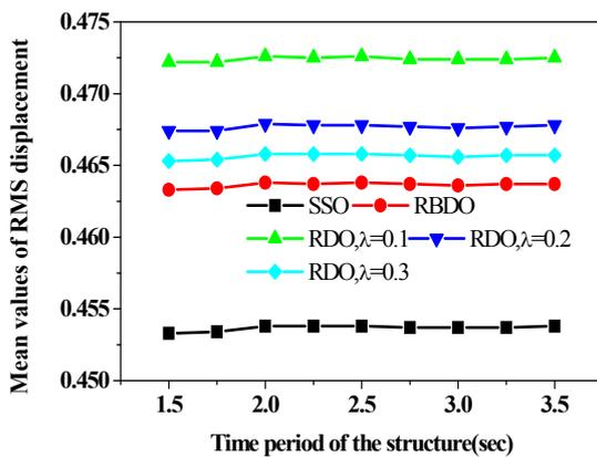
Fig. 12 The variation of the mean value of the rmsd of the primary structure with varying time period
