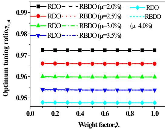
Fig. 8 The optimum tuning ratio with varying weight factor,  $\lambda$  for different mass ratio
