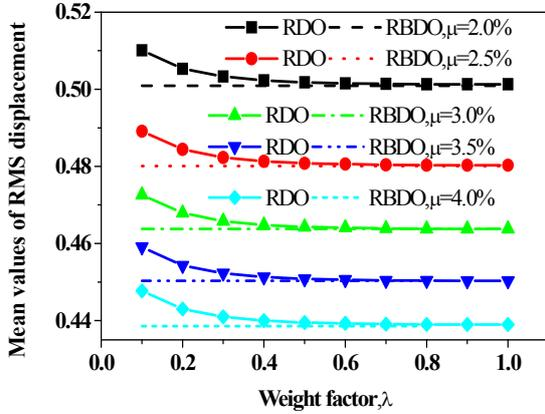
Fig. 6 The variation of the mean value of the rmsd of the primary structure with varying weight factor,  $\lambda$  for different mass ratio
