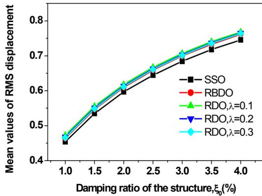
Fig. 10 The variation of the mean value of the rmsd of the primary structure with increasing damping ratio
