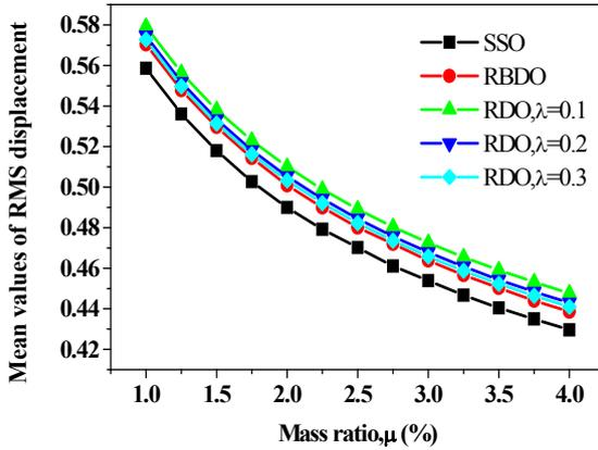
Fig. 2 The variation of the mean value of the rmsd of the primary structure with increasing mass ratio
