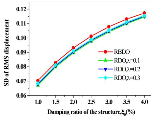
Fig. 11 The variation of the SD of the rmsd of the primary structure with increasing damping ratio
