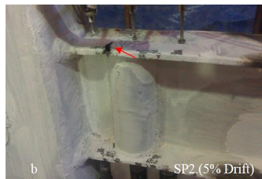
(b) Fracture in the right beam at 5% story drift
