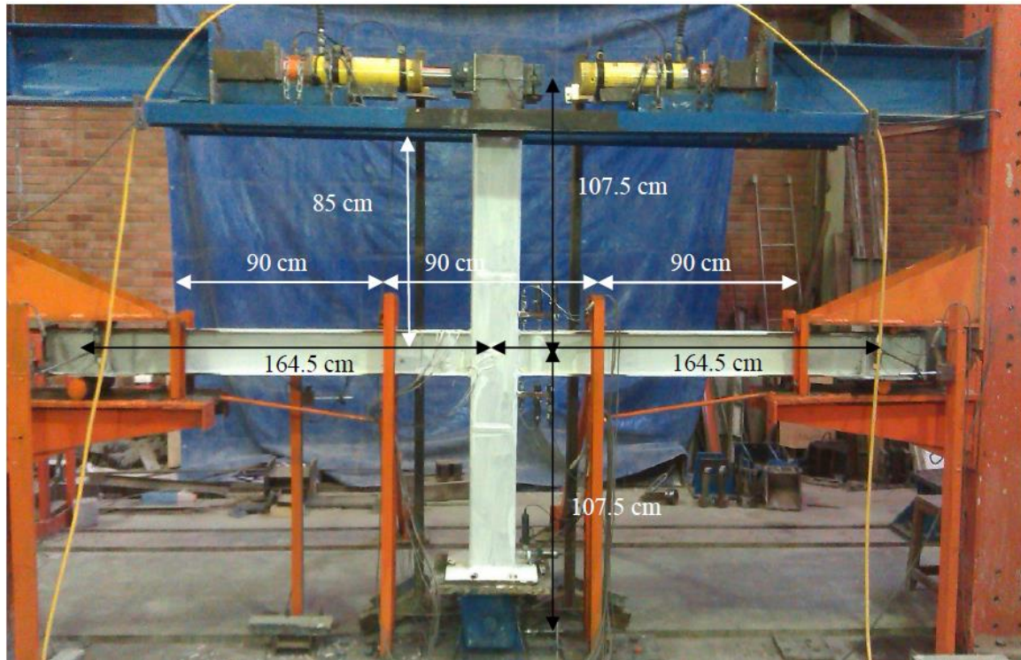
Fig. 3 Test setup configuration and overall dimensions of the specimens
