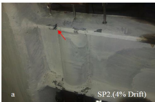
(a) Fracture in the right beam at 4% story drift
