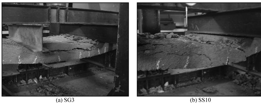
Fig. 11 Failure of specimen SG3 and SS10
