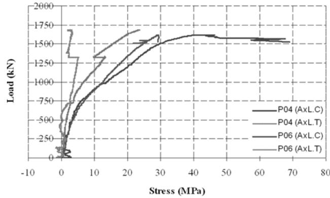
Fig. 15 Load versus stress (in strain gauges placed on strips)
