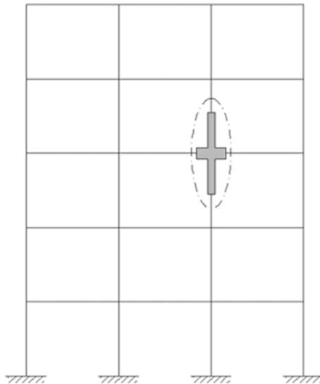
Fig. 3 Structure zone of a building simulated by specimens
