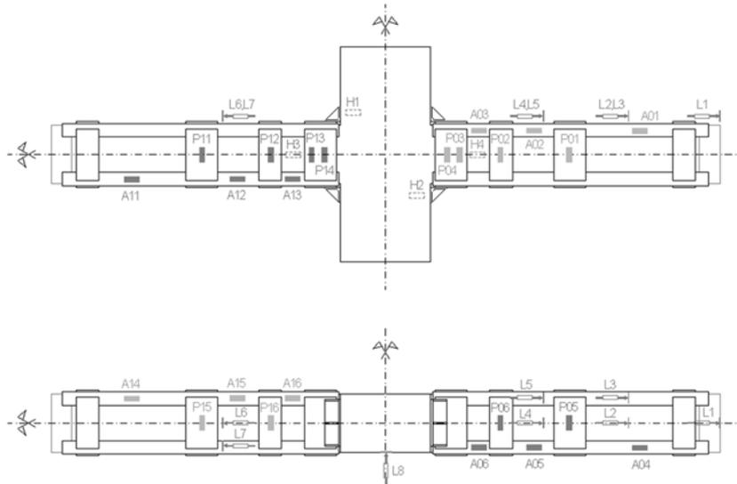
Fig. 8 Instrumentation of specimen AxL.C
