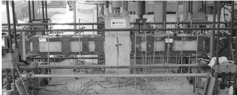
Fig. 10 General view of steel test frame with specimen ready for testing
