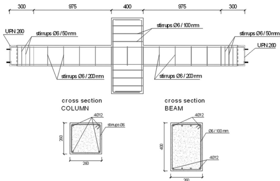
Fig. 4 Specimen geometry and reinforcement
