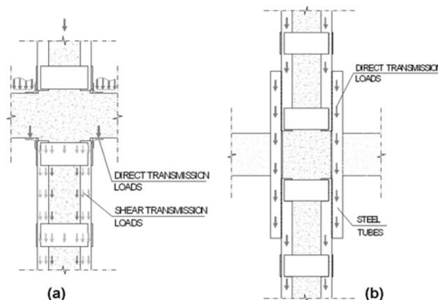
Fig. 2 Load transmission mechanisms
