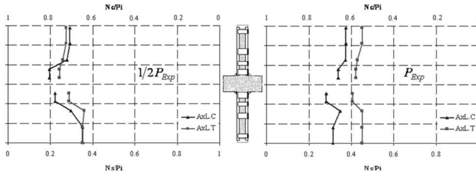
Fig. 14 Load distribution between column and steel cage along column axis
