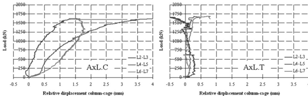
Fig. 13 Load versus relative displacement column-cage (slippage). Specimens AxL.C and AxL.T
