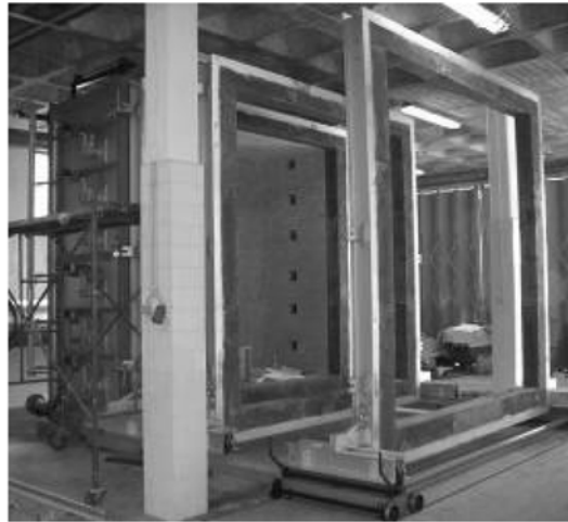
Fig. 1 Vertical furnace at the University of Aveiro, Portugal
