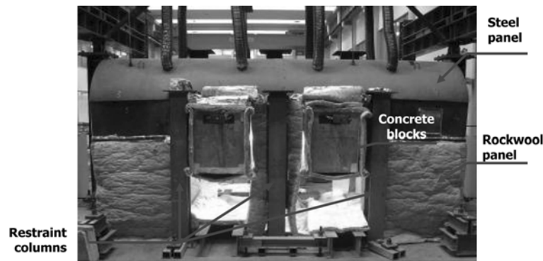
Fig. 13 General layout during a fire test
