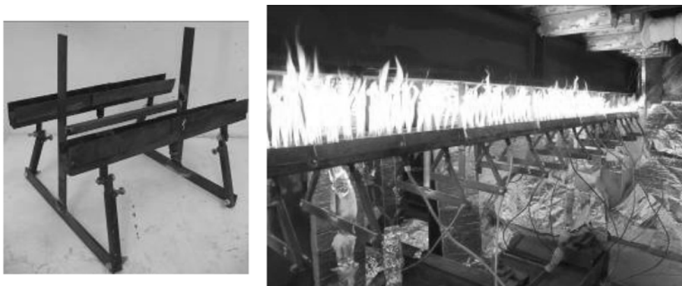
Fig. 5 a) Individual gas burner; b) Heating system
