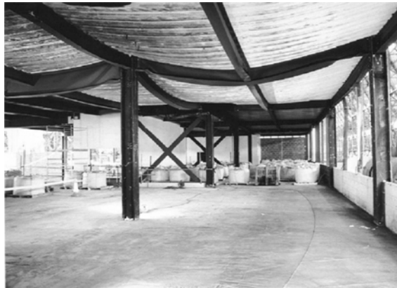
Fig. 1 Large deflections of restrained beams in Cardington experiments
