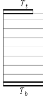
Fig. 6 Assumed cross-section distribution of temperature
