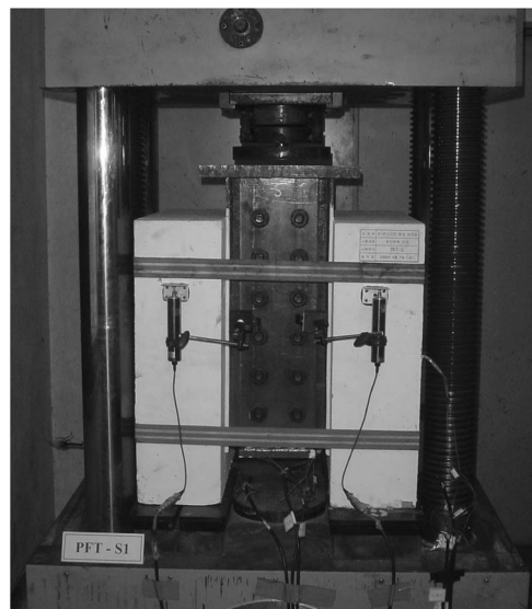
Fig. 4 Push-out test set-up
