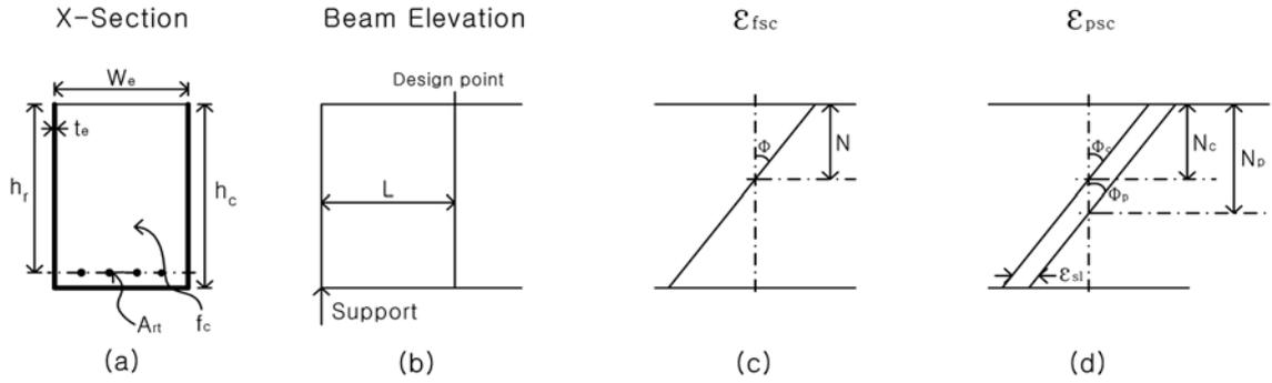
Fig. 2 Strain distribution in C-type MSC beam
