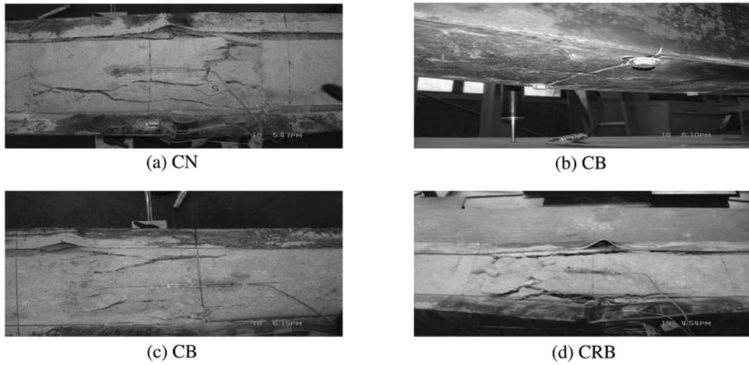
Fig. 7 Failure shape of C-type MSC beams
