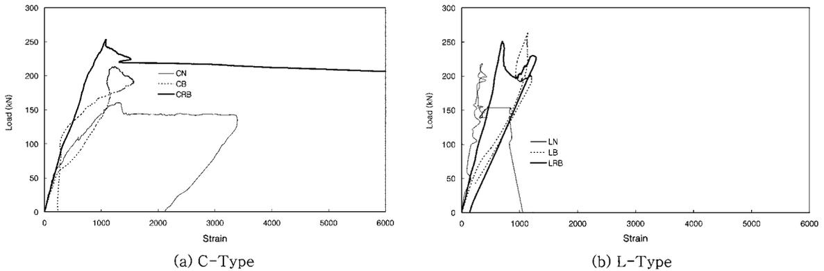
Fig. 11 Load strain of MSC beams (Bottom-fiber steel strain)
