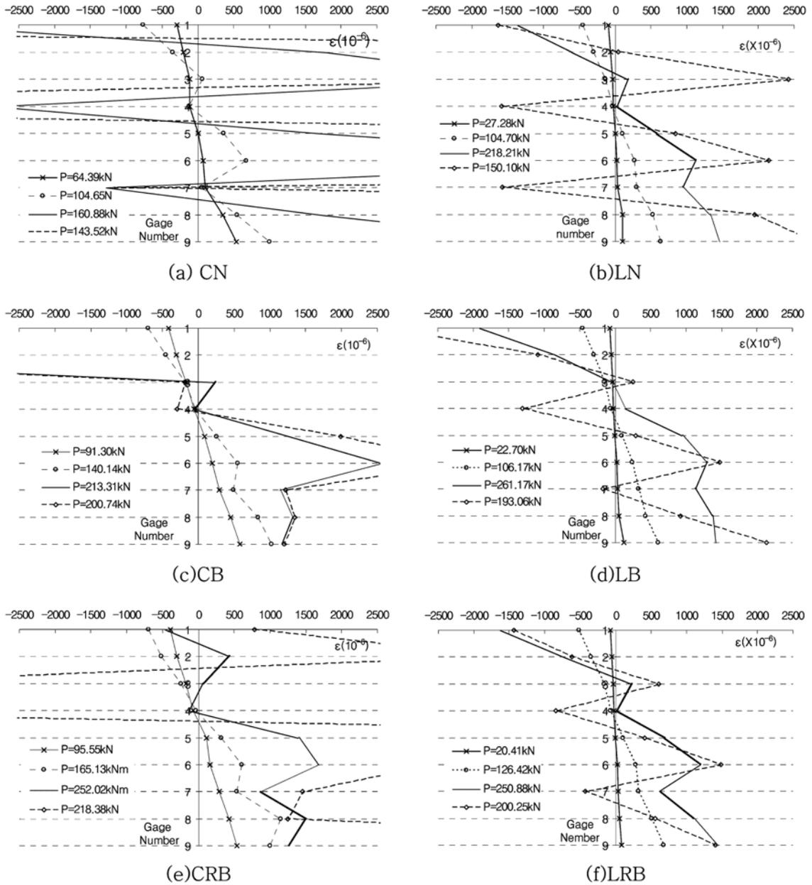
Fig. 12 Strain distribution of MSC beams according to gage number
