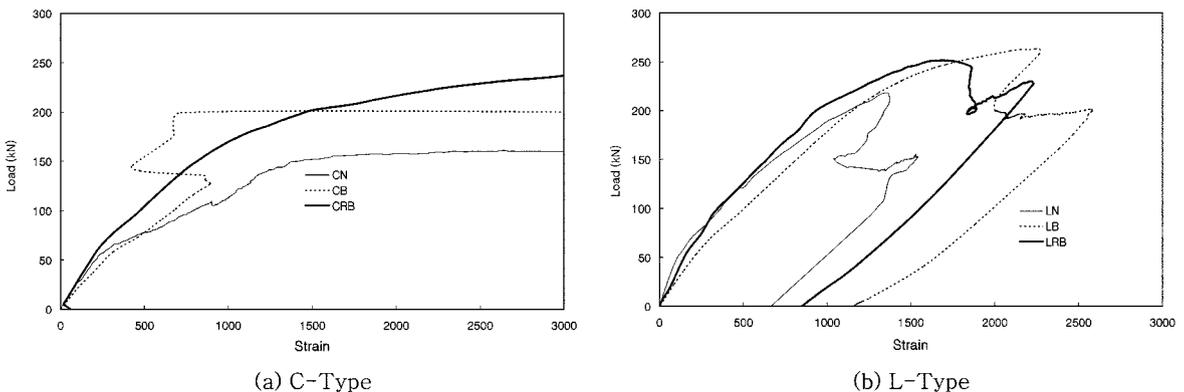
Fig. 10 Load strain of MSC beams (Top-fiber concrete strain)
