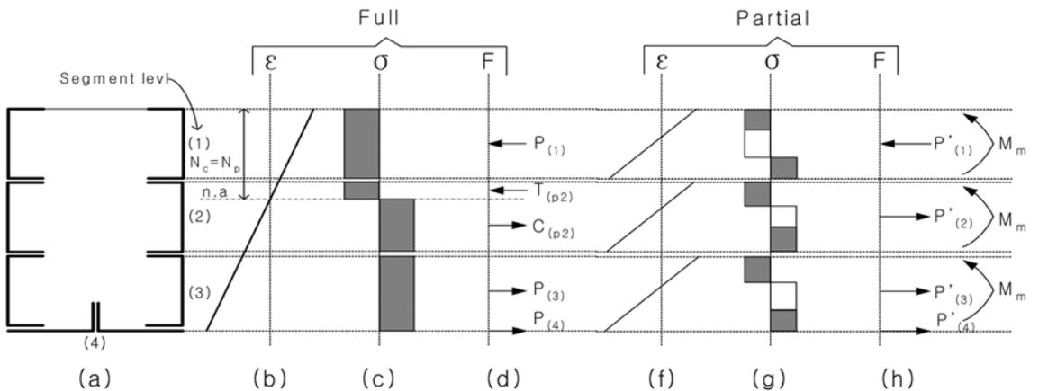
Fig. 4 Profile beam with shear connection
