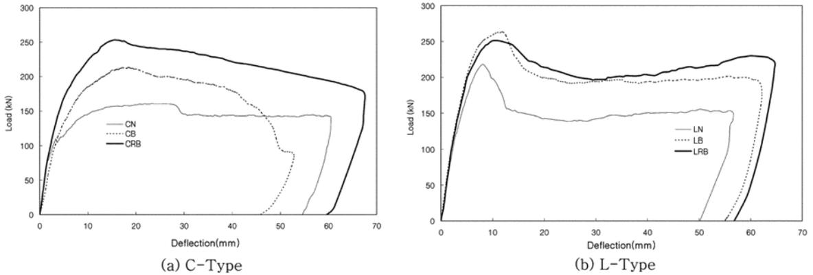
Fig. 9 Load deflection of MSC beams (midspan)
