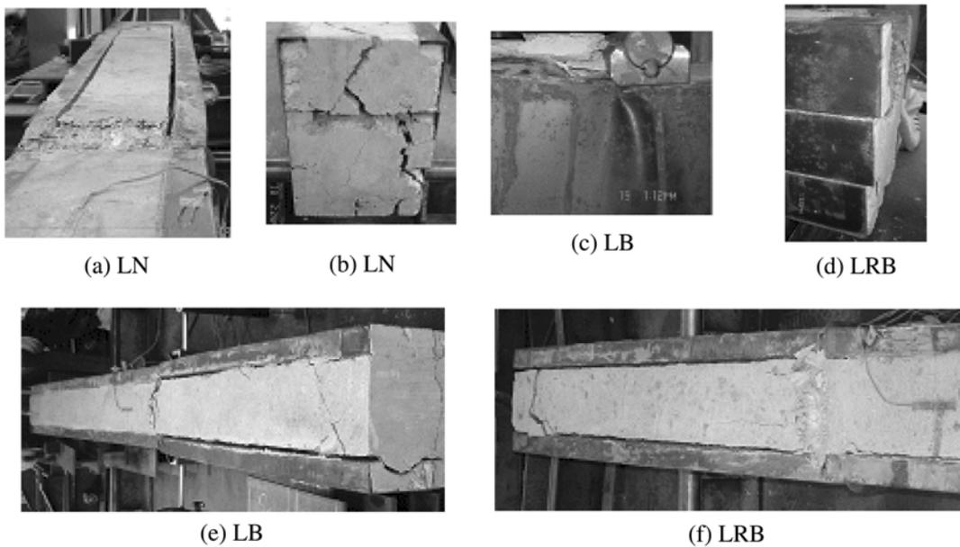
Fig. 8 Failure shape of lip-type MSC beams
