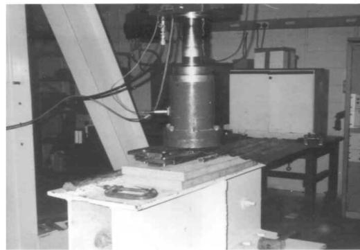
Fig. 3 Manufacture of model profiled sheets in a fly press
