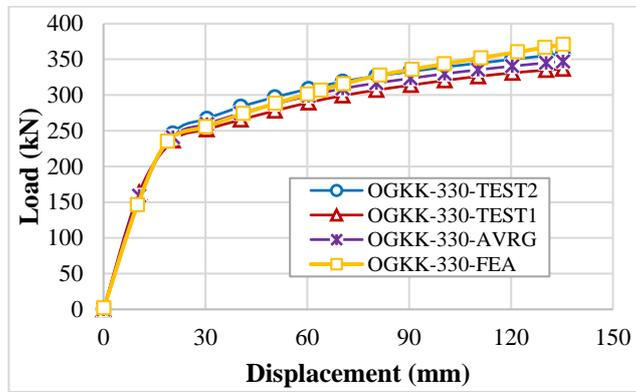
Fig. 21 Load-deflection curve for experimental and FEA results on OGKK\_330
