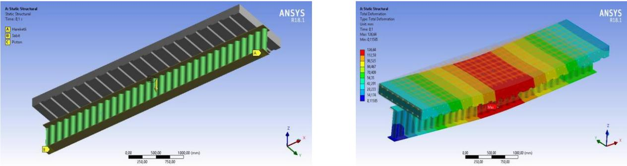
(a) Applying pressure (b) Deformation values
