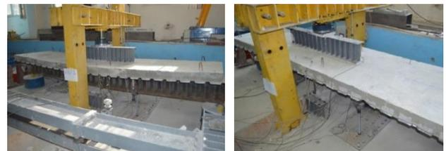
Fig. 9 Flexural bending on composite OGKK\_415
