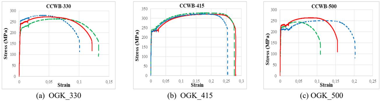
Fig. 15 Stress-strain graph of tensile tests of corrugated steel web beam specimens
