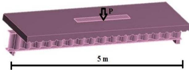
Fig. 3 Loading of 5-m span corrugated web beam
