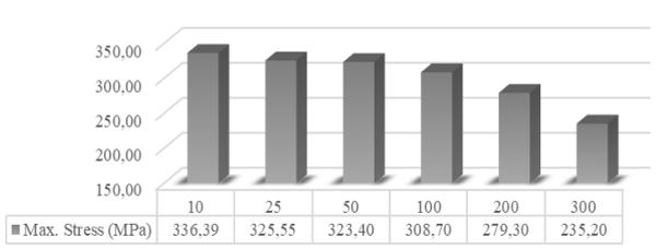
Fig. 16 Different mesh sizes and stress values
