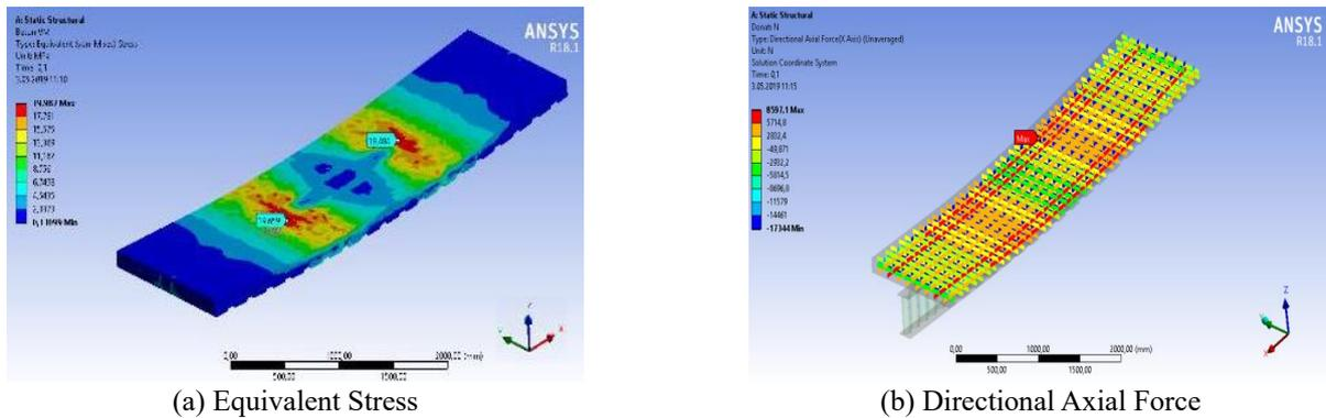
Fig. 24 Stress and Force Values on OGKK\_330 Slab and Reinforcement Mesh
