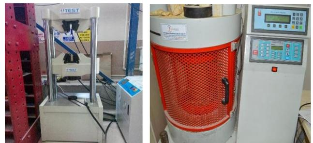
Fig. 14 Tension and compression tests on OGKK specimens
