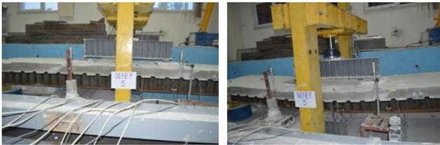
Fig. 6 Flexural Bending on Composite OGKK\_330
