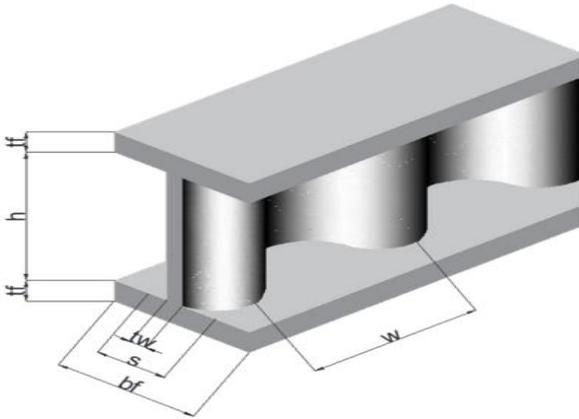
Fig. 1 Geometric properties of corrugated web beam
