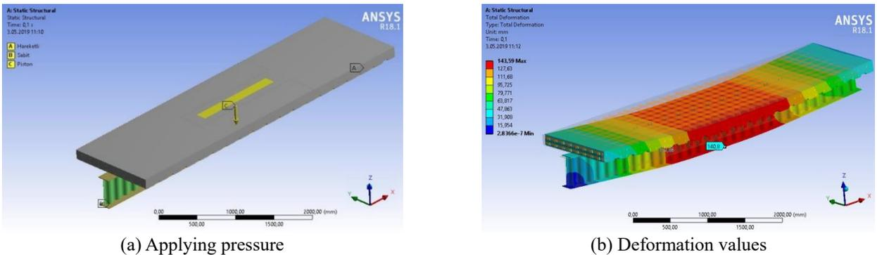
Fig. 22 Applying force and deformation values on OGKK\_415
