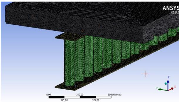
Fig. 17 Tetrahedron mesh model with 10-mm size
