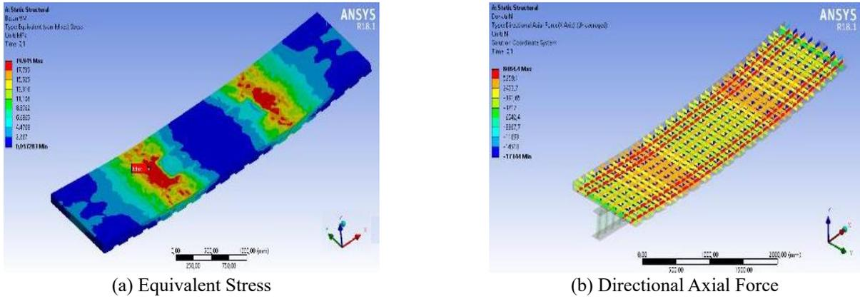
Fig. 20 Stress and force values on OGKK\_330 slab and reinforcement mesh
