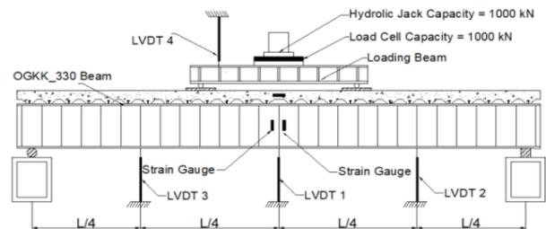
Fig. 8 Details of test set up for OGKK\_415 composite beams
