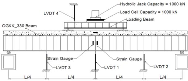
Fig. 5 Details of test set up for OGKK\_330 composite beams
