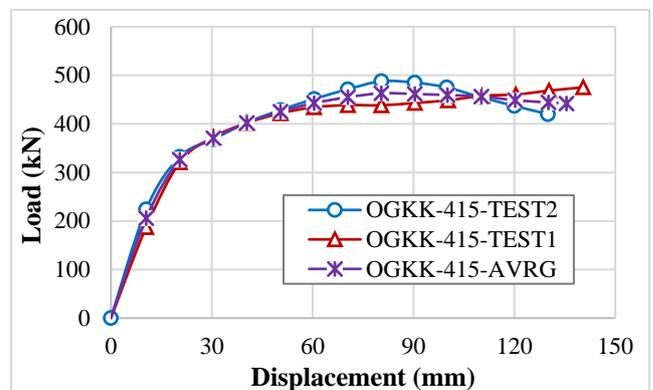
Fig. 10 The Load-deflection graphics for OGKK\_415
