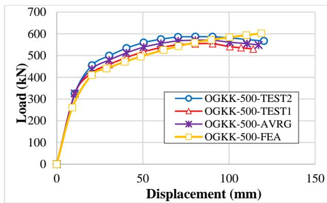
Fig. 29 Load-deflection curve for experimental and FEA results on OGKK\_500
