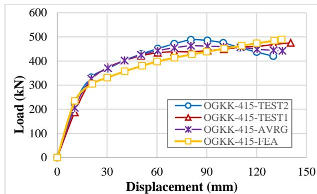
Fig. 25 Load-deflection curve for experimental and FEA results on OGKK\_415
