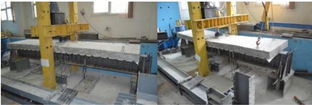
Fig. 12 Flexural bending on composite OGKK\_500 corrugated web beam
