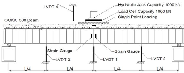
Fig. 11 Details of test set up for OGKK\_500 composite beams
