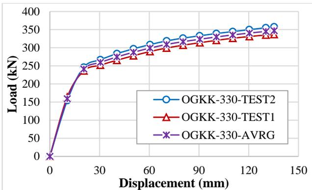
Fig. 7 The Load-deflection graphics for OGKK\_330
