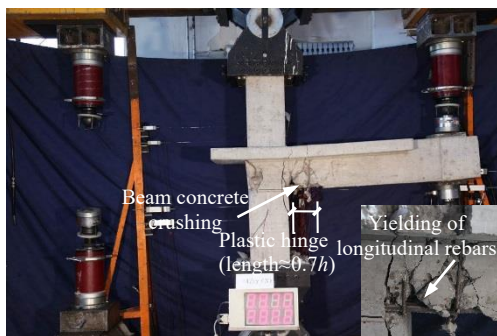
(e) J1-2 (Observed, Beam bending failure)
