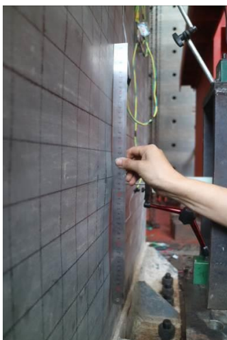
(a) Slight buckling on side N
