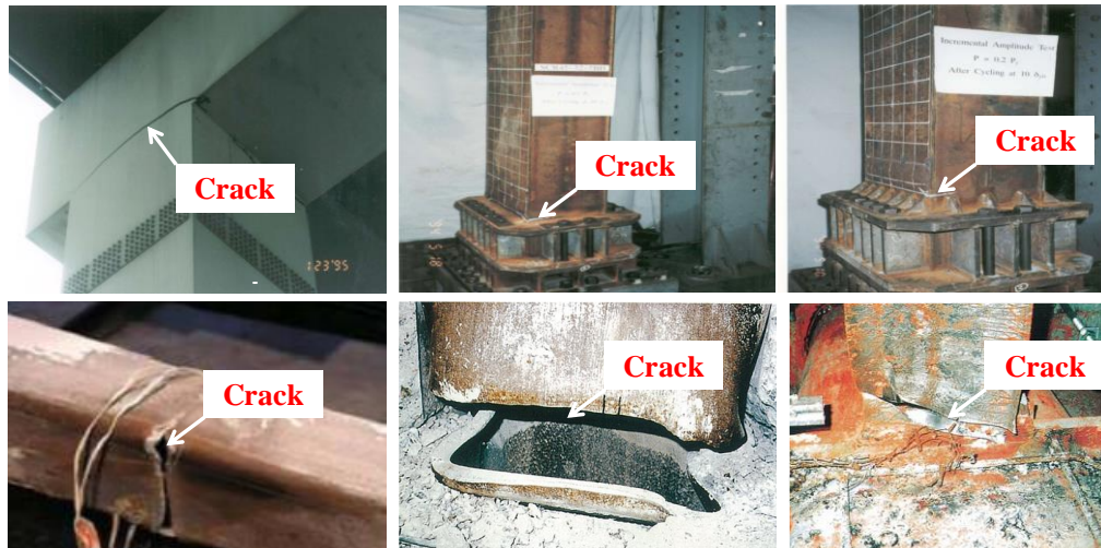
Fig. 1 Photos of crack of steel members in lab and practical engineering
