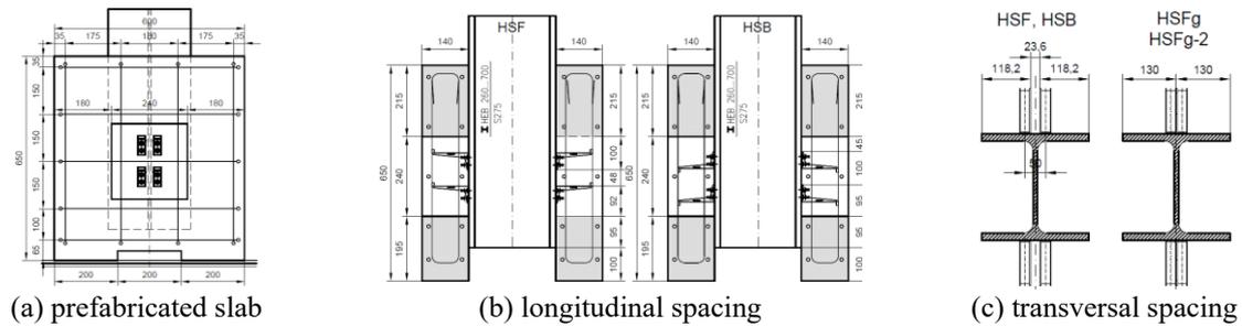
Fig. 2 Geometry of push-out specimens
