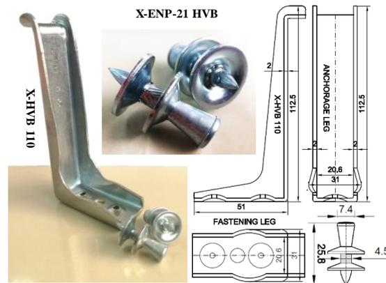
Fig. 1 Geometry of X-HVB 110 shear connector
