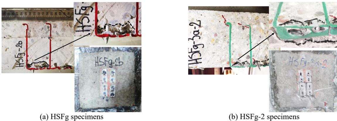
Fig. 12 Specimens after testing procedure – reduced distances between connectors
