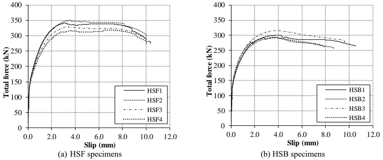
Fig. 7 Results of push-out tests – minimal distance between shear connectors
