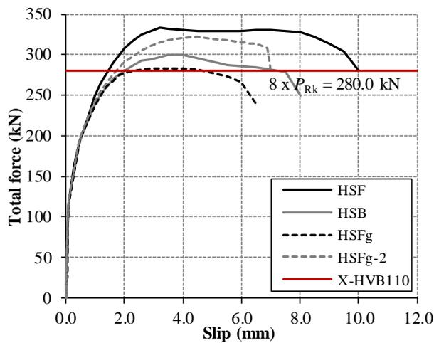
Fig. 9 Average results of push-out tests
