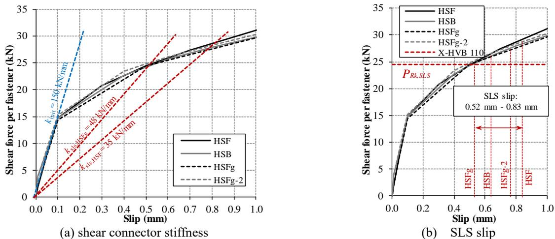
Fig. 10 Average results of push-out tests
