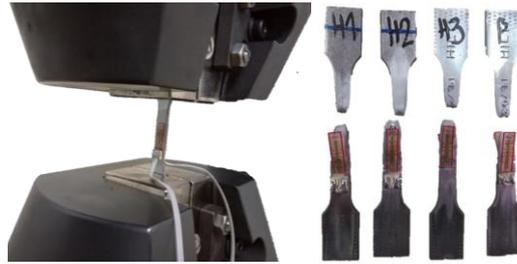
Fig. 5 Tensile test for flat coupons – shear connector
