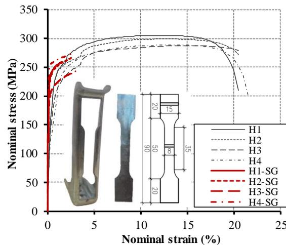
Fig. 6 Nominal stress-strain curves
