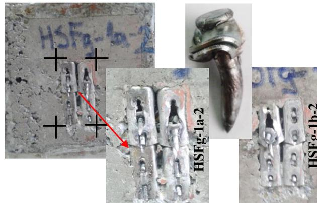
Fig. 13 Inappropriate installation of cartridge fired pins
