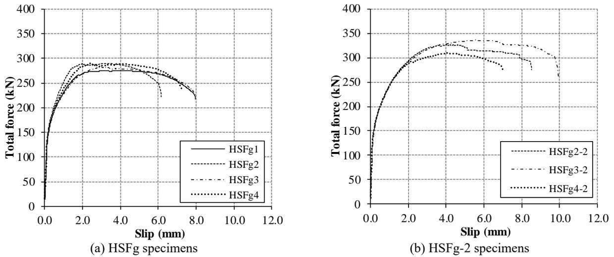
Fig. 8 Results of push-out tests – reduced distance between shear connectors
