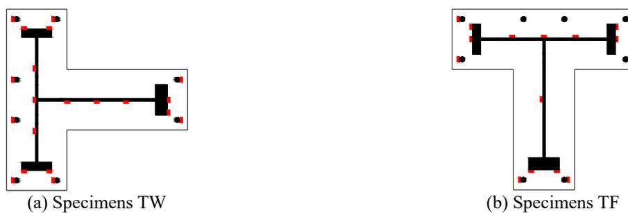
Fig. 12 Measurement points of strains for solid-web steel and longitudinal rebars
