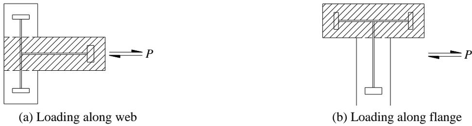
Fig. 23 The effective shear area of concrete within the section of SRC T-shaped column
