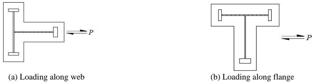
Fig. 24 The effective shear area of steel within the section of SRC T-shaped column
