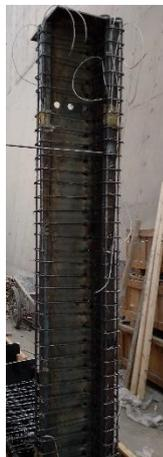
Fig. 7 Complete steel skeleton
