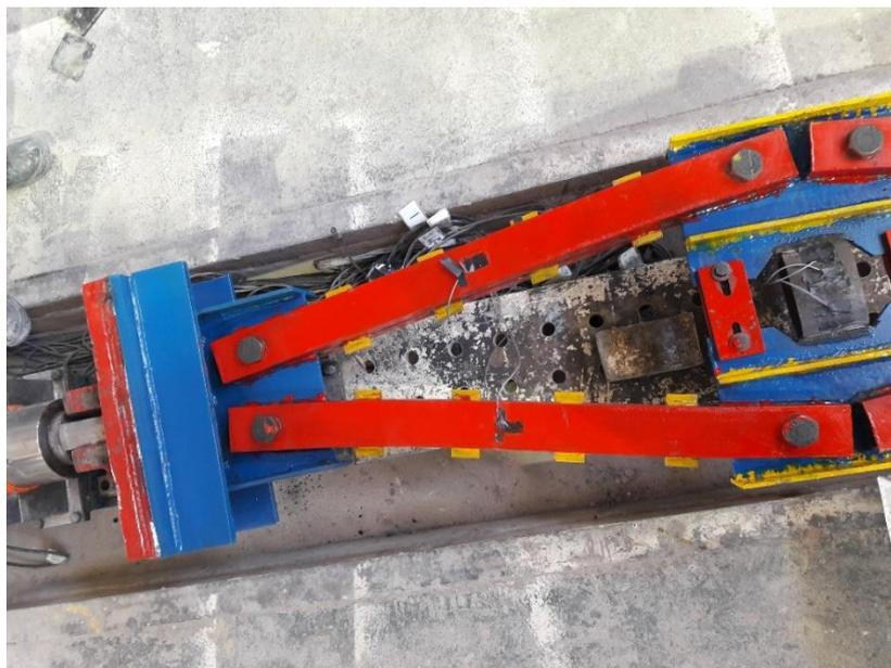
Fig. 11 Buckling of Diagonals
