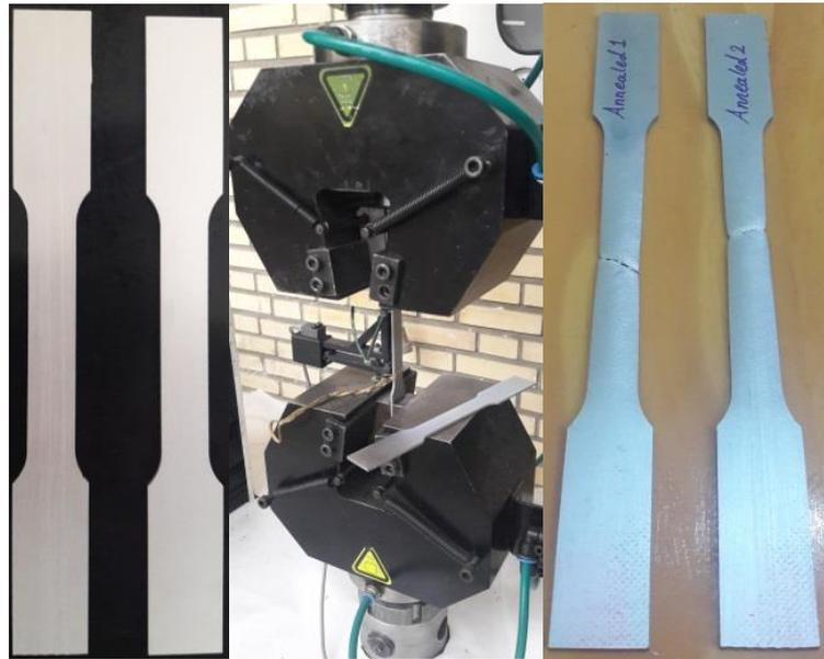
Fig. 3 Wire-cut specimens for tensile test and their positioning in the SANTAM machine (ASTM Standard E8/E8M-13a, 2013)
