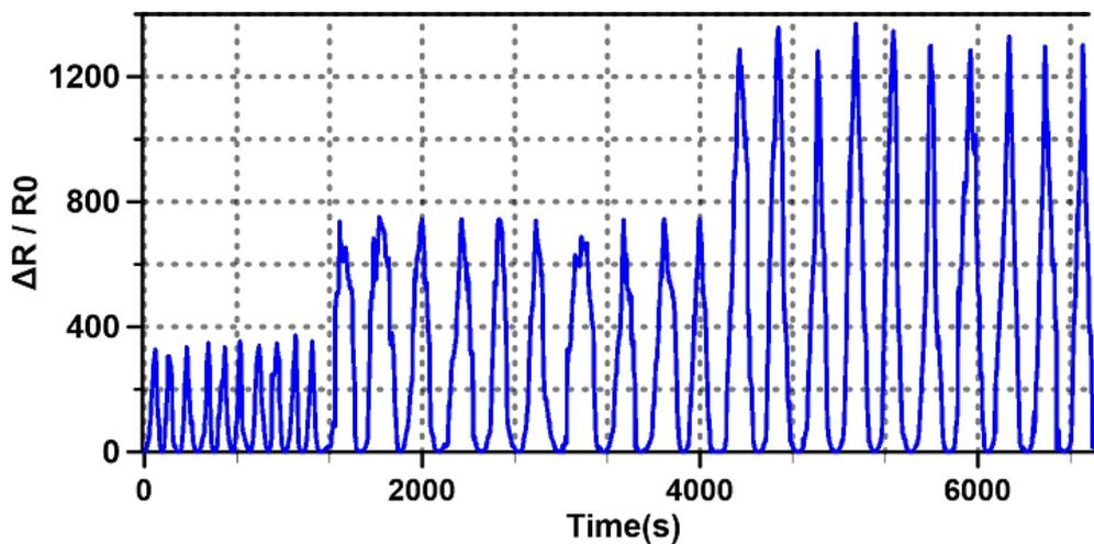
Fig. 3 Resistance changes over time at 80%, 100%, and 120%
