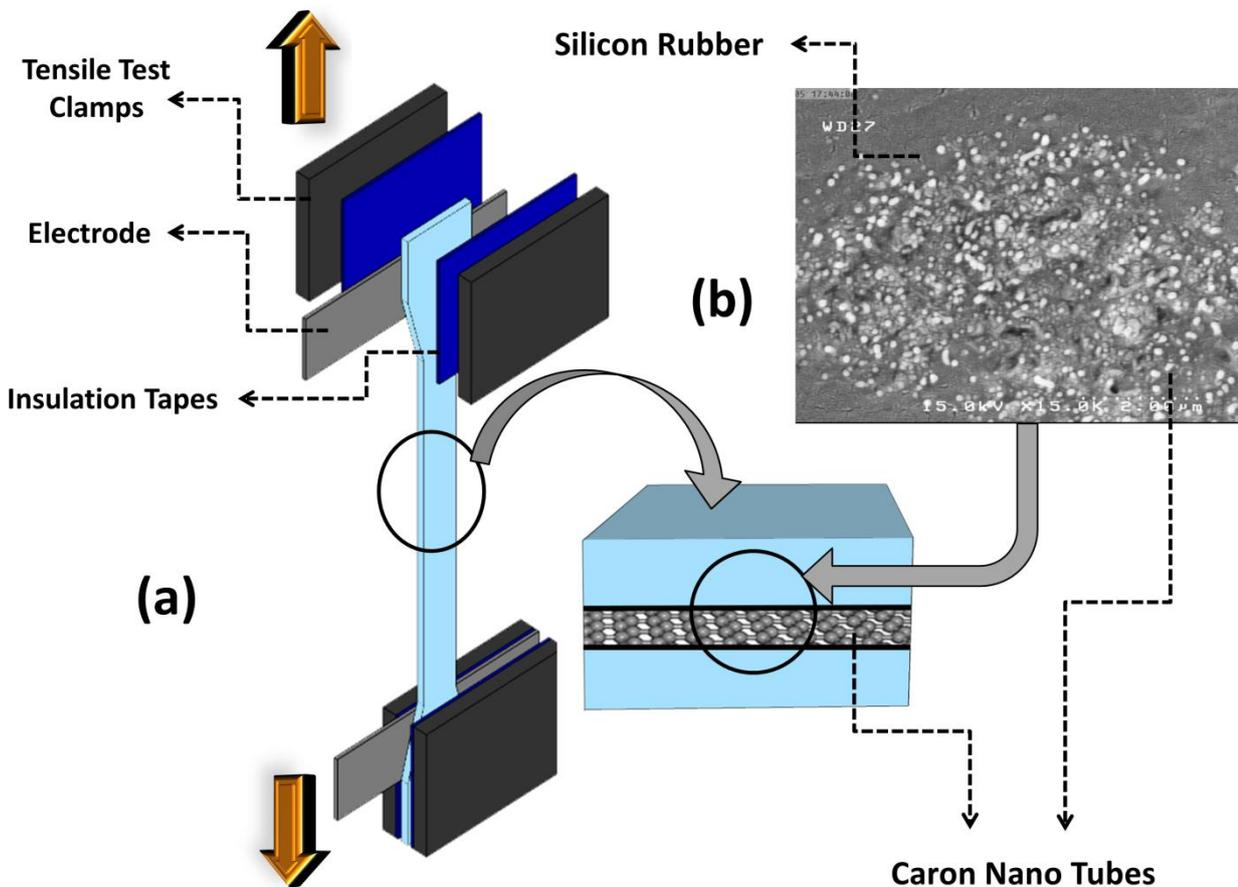
Fig. 1 Schematic view of the CNT/Silicon Rubber strain sensor installation in the Universal tensile testing fixtures while recording the performance by attaching the probes to two electrodes
