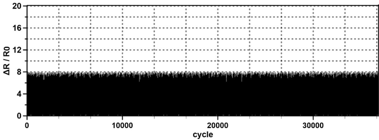
Fig. 4 Time/resistance changes during about 4,000 loading/unloading cycles at 4% strain value
