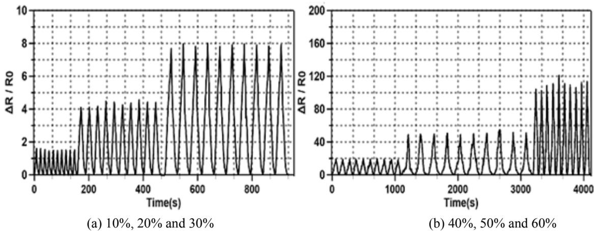
Fig. 2 Resistance changes over time at different strain values
