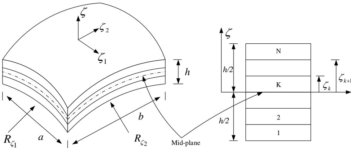
Fig. 2 Representation of shell panel type composite
