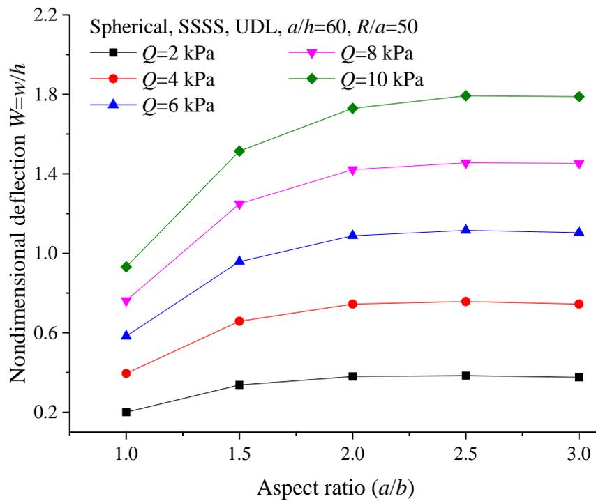
Fig. 5 Variation of non-dimensional non-linear deflection with aspect ratio ( $a/b$ )
