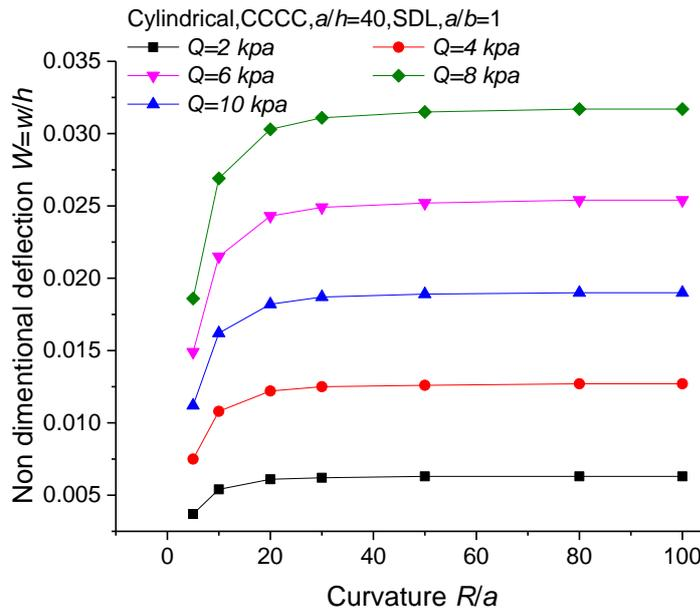
Fig. 6 Variation of non-dimensional non-linear deflection with curvature ( $R/a$ )
