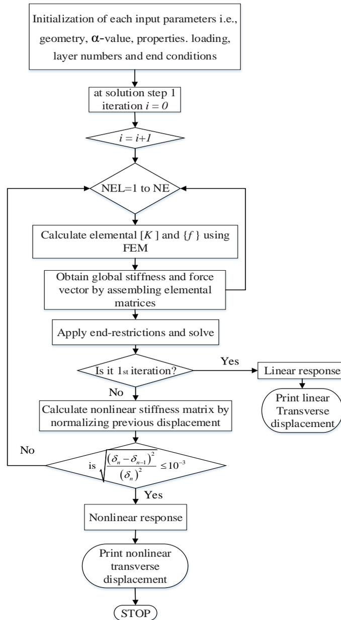
Fig. 3 Flowchart presentation for linear/nonlinear bending analysis
