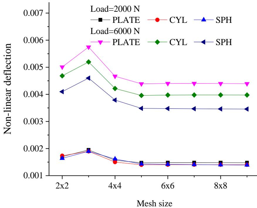
Fig. 4 Variation of non-dimensional non-linear deflection with the mesh size
