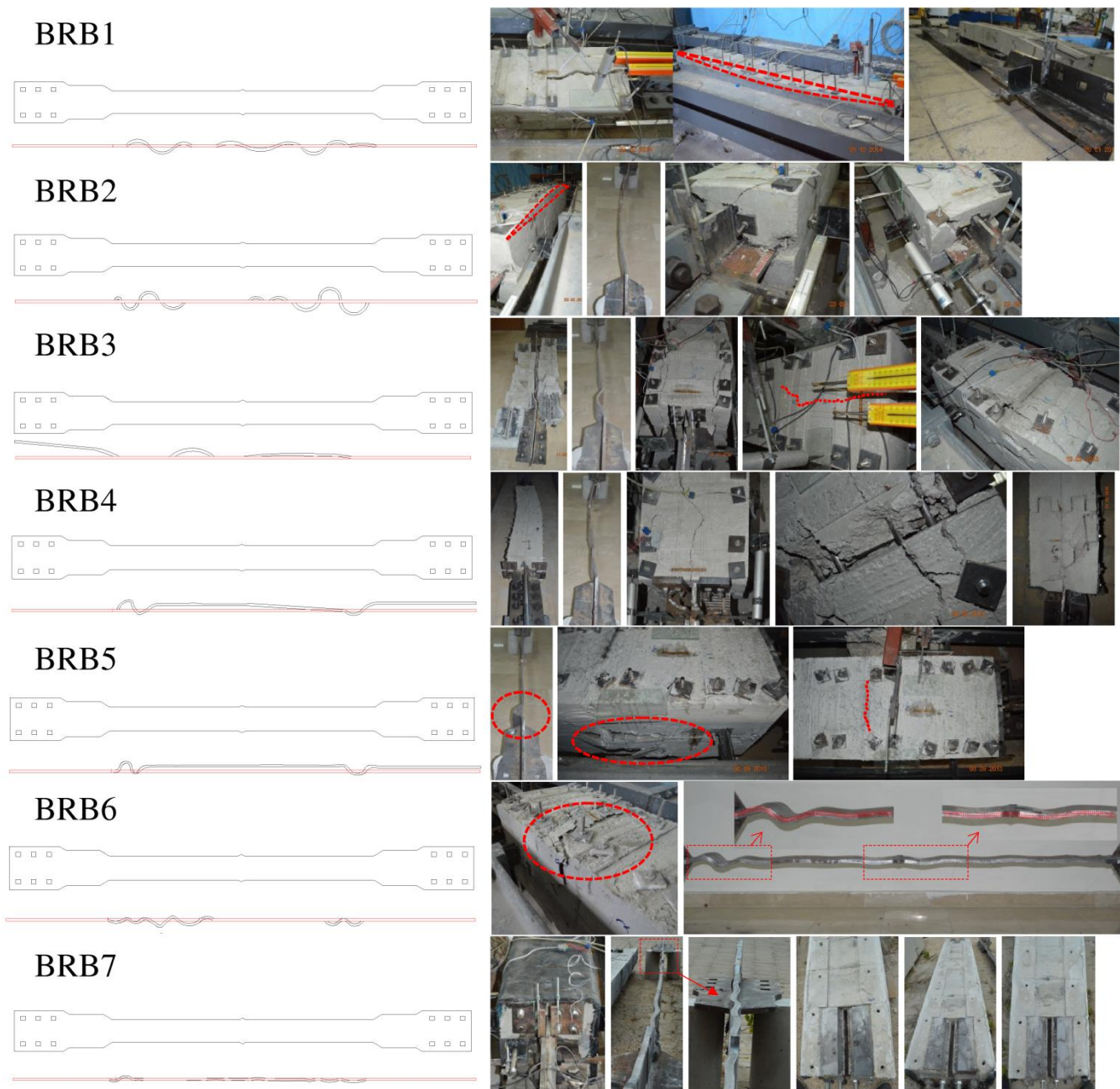
Fig. 10 Physical damage of the specimens BRB1 to 7.
