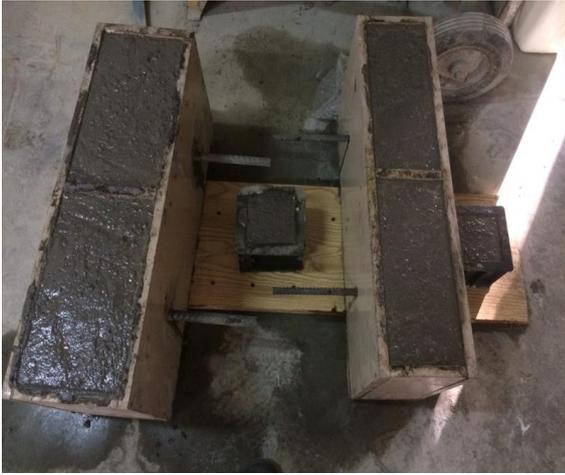
Fig. 4 Laboratory specimens prepared for pullout testing and compressive strength determination
