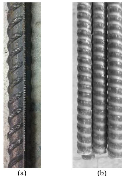
Fig. 1 The surface of the used steel (a) and GFRP (b) bars
