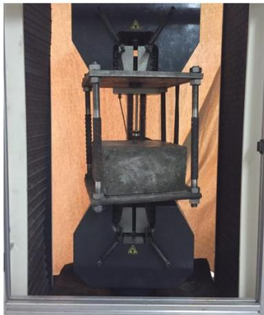
Fig. 5 Pull-out experimental set-up
