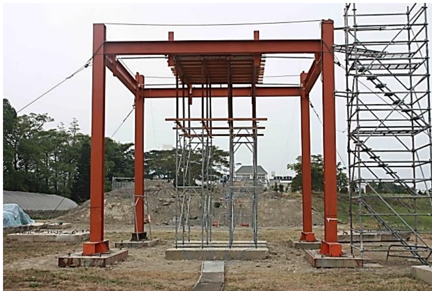
Fig. 7 Setup of the combined system of scaffolds and shores in the outdoor loading test on site
