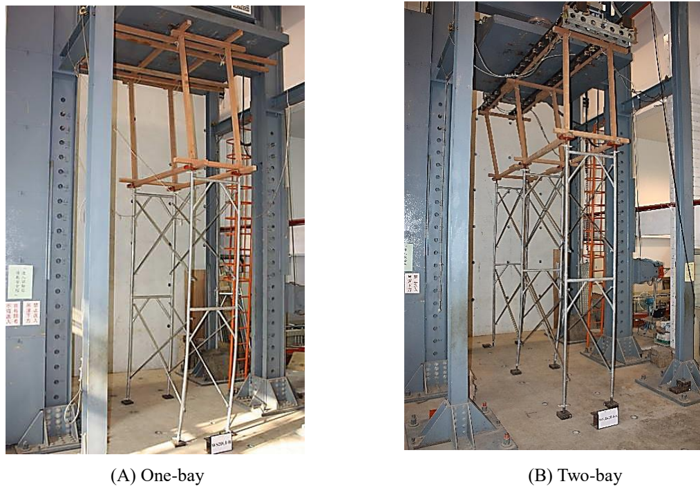
Fig. 13 Failure shapes of one-bay and two-bay combined system of scaffolds and shores in tests
