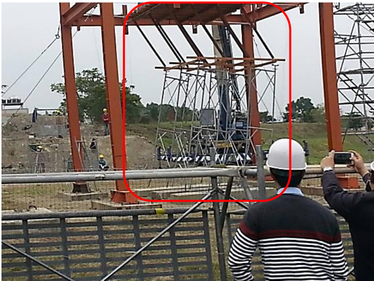
Fig. 24 No damage to components at collapse moment in combined system of scaffolds and shores in outdoor loading test
