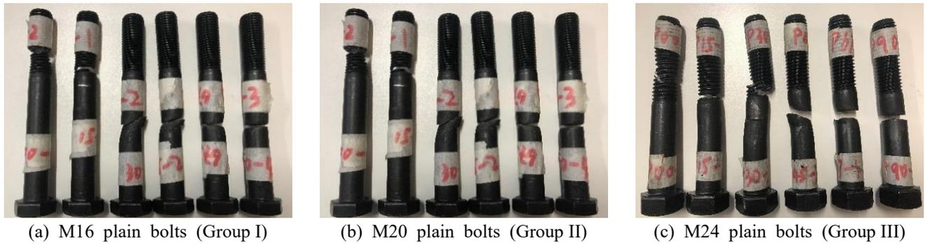
Fig. 6 Failure modes of plain bolts
