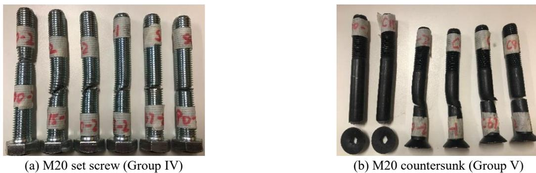
Fig. 8 Failure modes of set screw and countersunk bolts
