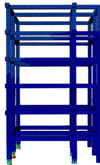
Fig. 24 Deformation of frame after inverse loading
