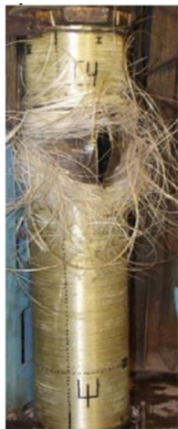
(a) Pipe after experiment test
