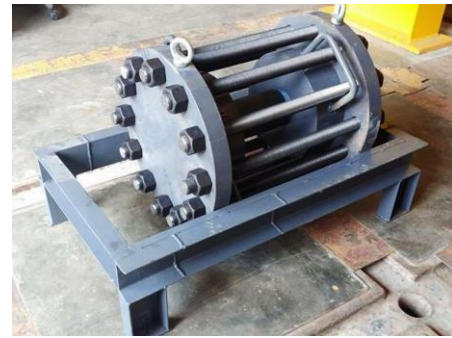
Fig. 16 Completed burst rig assembly
