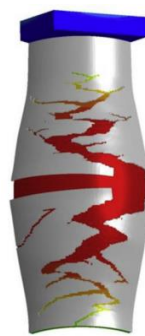
(b) Circumferential stresses from numerical analysis before failure
