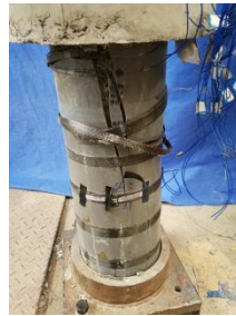
(b) Failure mode of PFCC column
