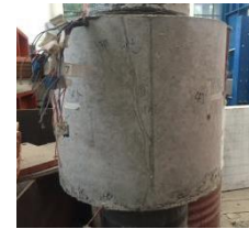
(c) Failure mode of joint zone
